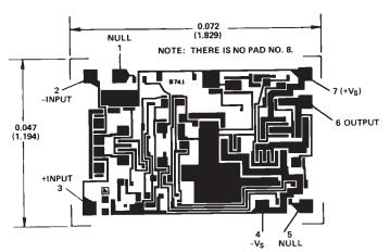
PAD NUMBERS CORRESPOND TO PIN NUMBERS FOR THE TO-99 8-PIN METAL PACKAGE.
