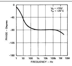
Figure 4. Open-Loop Phase Response vs. Frequency
