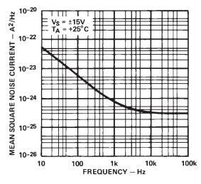
Figure 8. Input Noise Current vs. Frequency
