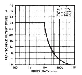
Figure 12. Output Voltage Swing vs. Frequency
