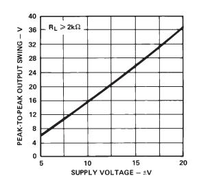
Figure 10. Output Voltage Swing vs. Supply Voltage
