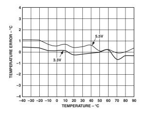
Figure 14. Typical Temperature Error @ 3.3 V and 5.5 V
