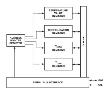
Figure 4. AD7414 Register Structure
