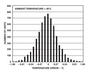
Figure 15. Ambient Temperature Error @ 3 V
