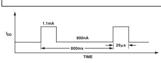
Figure 11. Mode 2 Power Dissipation
