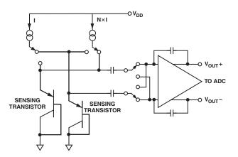
Figure 3. Temperature Measurement Technique
