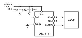
Figure 2. Typical Connection Diagram
