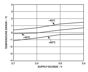
Figure 13. Typical Temperature Error vs. Supply for One Part
