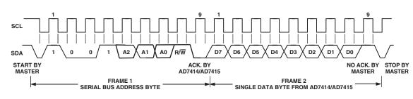
Figure 8. Reading a Single Byte of Data from a Selected Register
