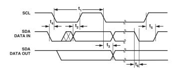
Figure 1. Diagram for Serial Bus Timing
