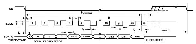
Figure 1. Serial Interface Timing Diagram
