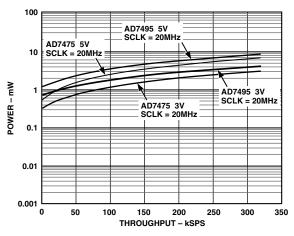
Figure 18. AD7495 Power vs. Throughput for Partial Power-Down
