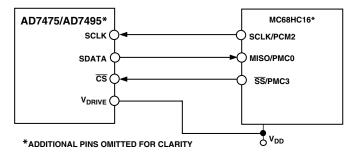
Figure 25. Interfacing to the MC68HC16
