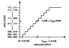
Figure 6. AD7475/AD7495 Transfer Characteristic
