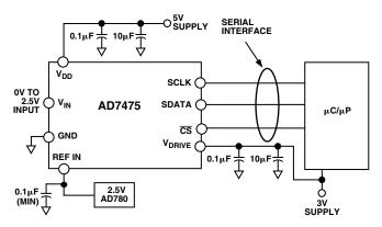
Figure 7. AD7475 Typical Connection Diagram
