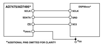
Figure 24. Interfacing to the DSP56xxx
