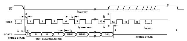
Figure 21. Serial Interface Timing Diagram-Conversion Termination
