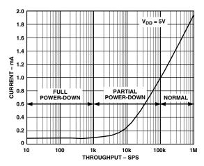
Figure 19. Typical AD7495 Current vs. Throughput
