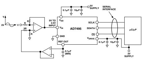
Figure 8. AD7495 Typical Connection Diagram
