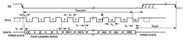
Figure 20. Serial Interface Timing Diagram
