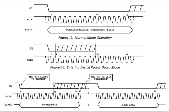
Figure 15. Exiting Partial Power-Down Mode
