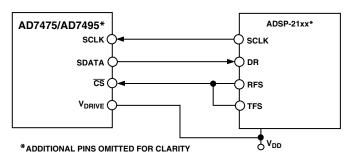
Figure 23. Interfacing to the ADSP-21xx
