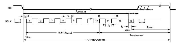
Figure 2. Serial Interface Timing Example
