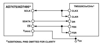
Figure 22. Interfacing to the TMS320C5x/C54x
