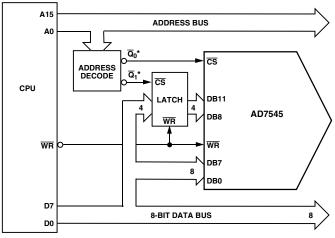
$\overline{*}$   $\overline{Q}_0$  = DECODED ADDRESS FOR DAC  $\overline{Q}_1$  = DECODED ADDRESS FOR LATCH
