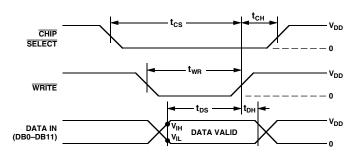
Write Cycle Timing Diagram
