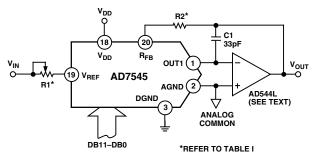
Figure 4. Unipolar Binary Operation
