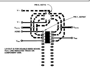
Figure 10. Suggested Layout for Circuit of Figure 4
