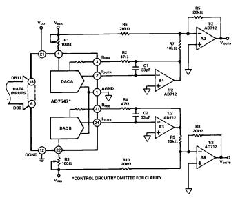
Figure 5. Bipolar Operation (Offset Binary Coding)
