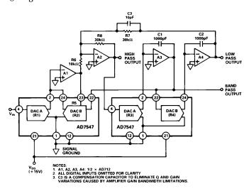
Figure 6. Programmable State Variable Filter
