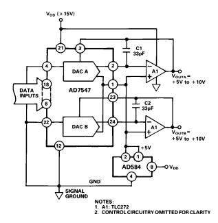
Figure 7. AD7547 Single Supply Operation
