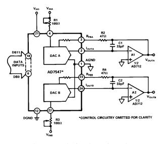
Figure 4. Unipolar Binary Operation
