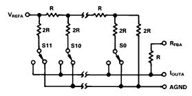
Figure 2. Simplified Circuit Diagram for DAC A
