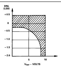
Figure 9. Differential Nonlinearity vs. Reference Voltage for Circuit of Figure 8.  $V_{DD}$  = 15 V. Shaded Area Shows Range of Values of Differential Nonlinearity that Typically Occur for L, C and U Grades
