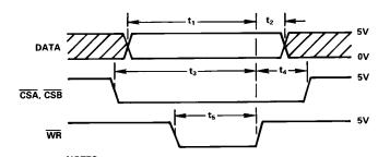
NOTES 1. ALL INPUT SIGNAL RISE AND FALL TIMES MEASURED FROM 10% TO 90% OF +5V. t, =  $t_f$  = 20ns. 2. TIMING MEASUREMENT REFERENCE LEVEL IS  $\frac{V_{H}+V_{IL}}{2}$
