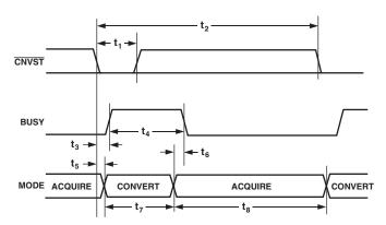
Figure 11. Basic Conversion Timing
