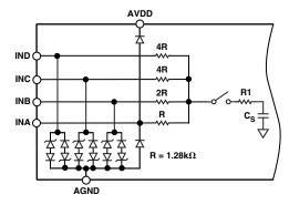
Figure 6. Simplified Analog Input
