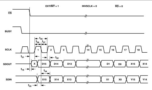
Figure 19. Slave Serial Data Timing for Reading (Read after Convert)
