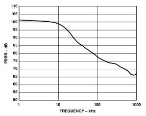
Figure 9. PSRR vs. Frequency
