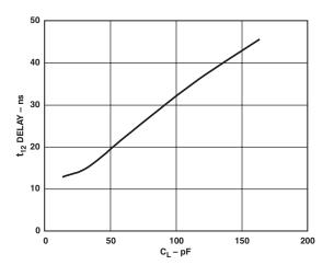
TPC 12. Typical Delay vs. Load Capacitance, C<sub>L</sub>
