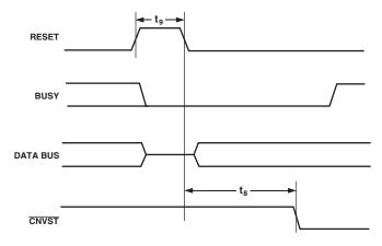
Figure 12. RESET Timing
