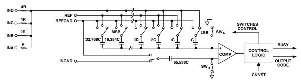
Figure 3. ADC Simplified Schematic
