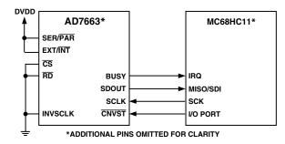
Figure 22. Interfacing the AD7663 to SPI Interface
