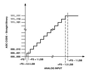
Figure 4. ADC Ideal Transfer Function
