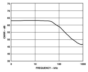
Figure 7. Analog Input CMRR vs. Frequency
