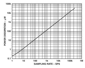
Figure 10. Power Dissipation vs. Sample Rate
