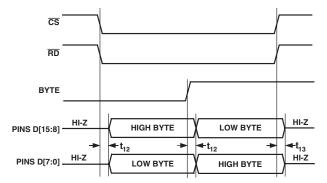
Figure 16. 8-Bit Parallel Interface
