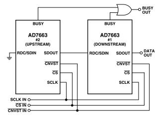
Figure 20. Two AD7663s in a Daisy-Chain Configuration
