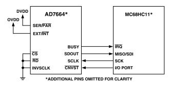
Figure 21. Interfacing the AD7664 to SPI Interface
