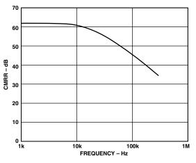
Figure 7. Analog Input CMR vs. Frequency
