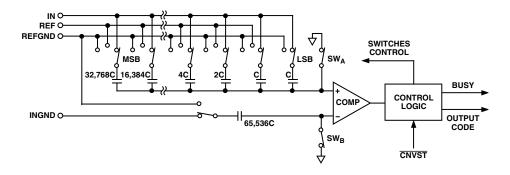
Figure 3. ADC Simplified Schematic
