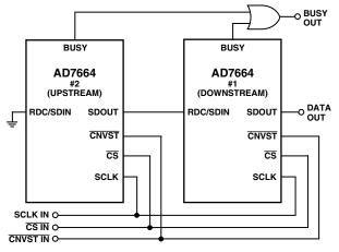
Figure 19. Two AD7664s in a "Daisy-Chain" Configuration
