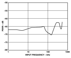
Figure 9. PSRR vs. Frequency
