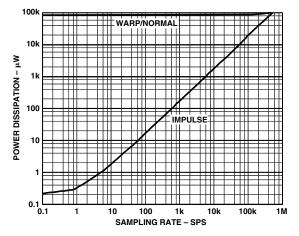
Figure 10. Power Dissipation vs. Sample Rate
