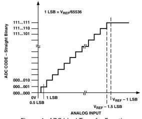
Figure 4. ADC Ideal Transfer Function
