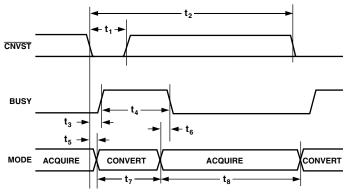
Figure 11. Basic Conversion Timing
