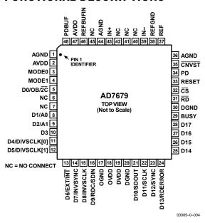
Figure 4. 48-Lead LQFP and 48-Lead LFCSP (ST-48 and CP-48)
