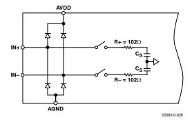
Figure 26. Simplified Analog Input
