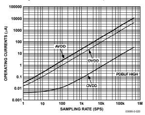
Figure 19. Operating Current vs. Sampling Rate
