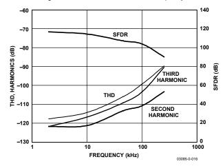
Figure 15. THD, SFDR, and Harmonics vs. Frequency
