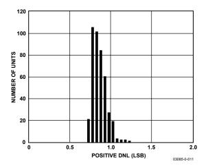
Figure 11. Typical Positive DNL Distribution (424 Units)
