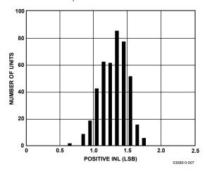
Figure 7. Typical Positive INL Distribution (424 Units)
