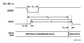
Figure 34. Master Parallel Data Timing for Reading (Continuous Read)
