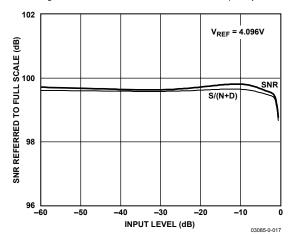
Figure 16. SNR and S/(N+D) vs. Input Level
