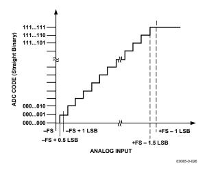
Figure 24. ADC Ideal Transfer Function
