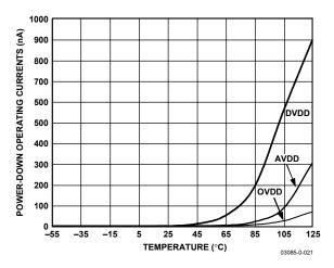
Figure 20. Power-Down Operating Currents vs. Temperature
