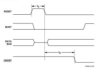
Figure 33. RESET Timing
