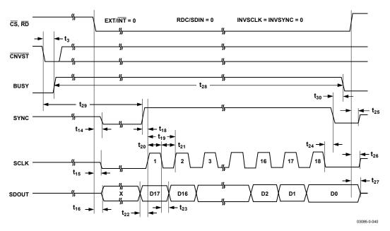
Figure 38. Master Serial Data Timing for Reading (Read after Convert)
