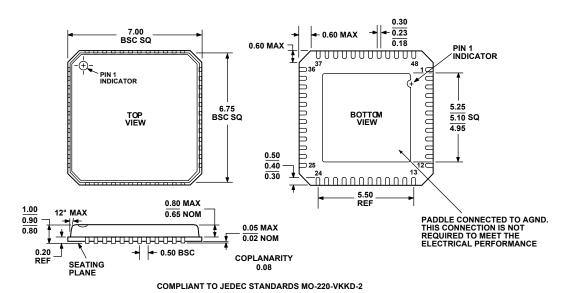
Figure 45. 48-Lead Frame Chip Scale Package [LFCSP] (CP-48) (Dimensions shown in millimeters)
