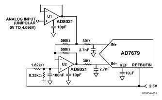
Figure 29. Single-Ended-to-Differential Driver Circuit (Internal Reference Buffer Used)
