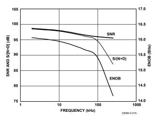
Figure 14. SNR, S/(N+D), and ENOB vs. Frequency
