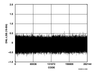
Figure 8. Differential Nonlinearity vs. Code
