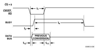
Figure 36. Slave Parallel Data Timing for Reading (Read during Convert)
