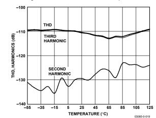
Figure 18. THD and Harmonics vs. Temperature
