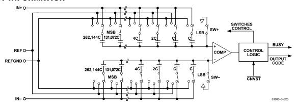
Figure 23. ADC Simplified Schematic
