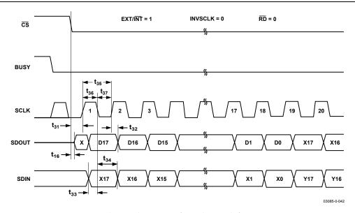
Figure 40. Slave Serial Data Timing for Reading (Read after Convert)
