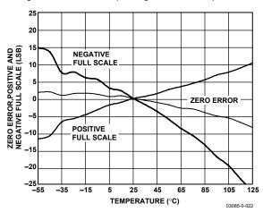
Figure 21. Zero Error Positive and Negative Full Scale vs. Temperature
