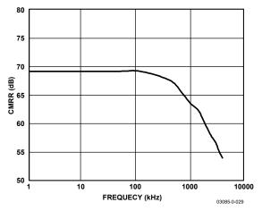
Figure 27. Analog Input CMRR vs. Frequency
