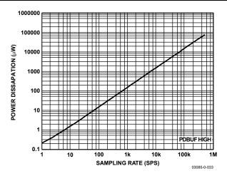
Figure 31. Power Dissipation vs. Sample Rate
