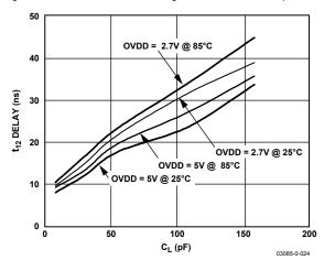
Figure 22. Typical Delay vs. Load Capacitance CL
