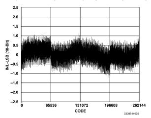
Figure 5. Integral Nonlinearity vs. Code
