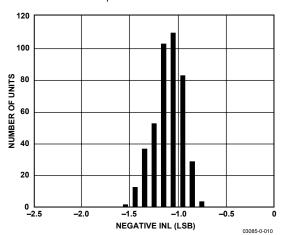
Figure 10. Typical Negative INL Distribution (424 Units)
