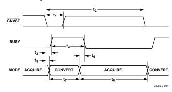
Figure 32. Basic Conversion Timing
