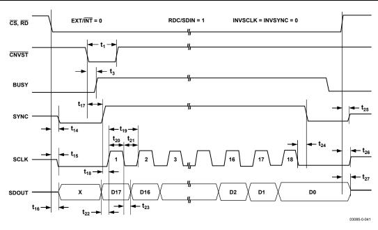
Figure 39. Master Serial Data Timing for Reading (Read Previous Conversion during Convert)
