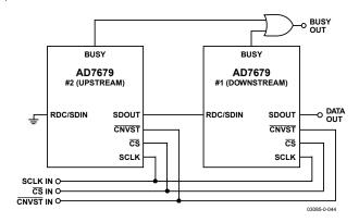
Figure 42. Two AD7679s in a Daisy-Chain Configuration
