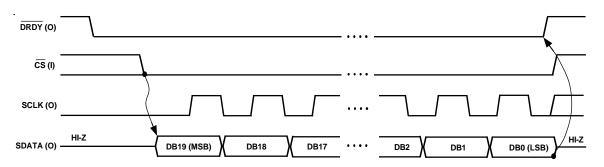
Figure 17. Timing Diagram for the SEC Mode
