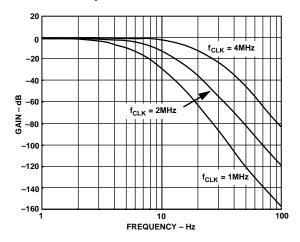
Figure 9. Frequency Response of AD7703 Filter
