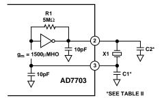
Figure 11. On-Chip Gate Oscillator
