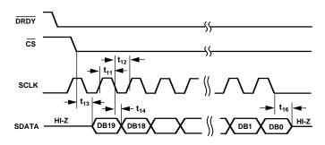
Figure 5b. SEC Mode Timing Diagram
