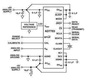
Figure 7. Typical System Connection Diagram
