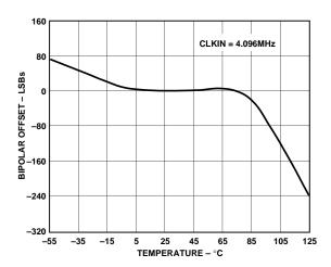
Figure 13. Typical Bipolar Offset vs. Temperature after Calibration at +25°C
