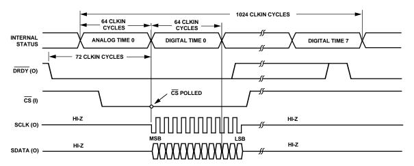
Figure 15. Timing Diagram for SSC Data Transmission Mode
