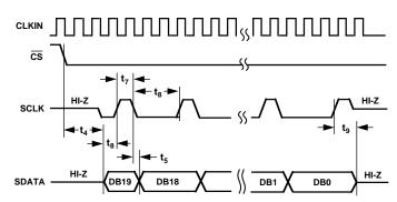
Figure 6. SSC Mode Timing Diagram
