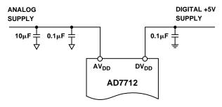
Figure 10. Recommended Decoupling Scheme
