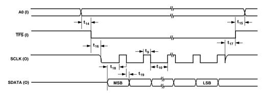
Figure 12. Self-Clocking Mode, Control/Calibration Register Write Operation
