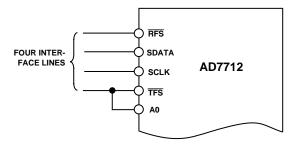
Figure 15. Simplified Interface with TFS Connected to A0
