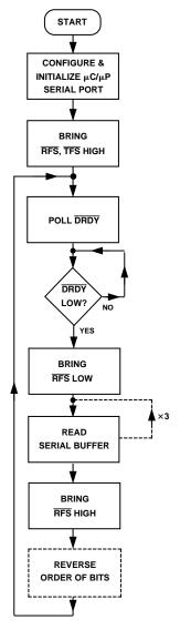
Figure 16. Flowchart for Continuous Read Operations to the AD7712
