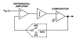
Figure 5. Basic Charge-Balancing ADC
