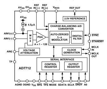
port. The AD7712 also contains self-calibration, system calibration and background calibration options and also allows the user to read and to write the on-chip calibration registers.
