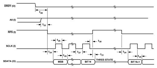
Figure 13b. External Clocking Mode, Output Data Read Operation (RFS Returns High During Read Operation)
