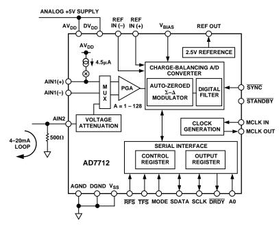
Figure 21. 4–20 mA Loop Measurement Using the AD7712
