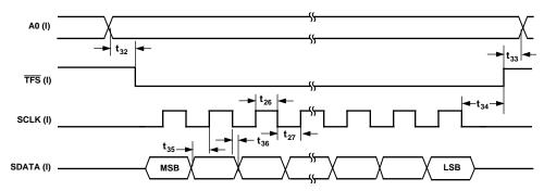
Figure 14a. External Clocking Mode, Control/Calibration Register Write Operation
