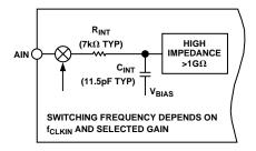
Figure 7. AIN1 Input Impedance
