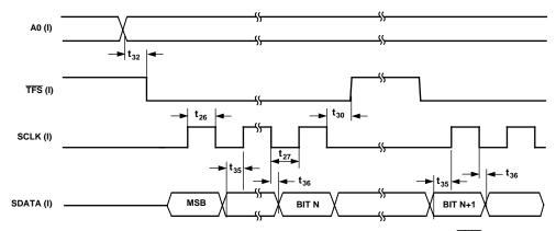
Figure 14b. External Clocking Mode, Control/Calibration Register Write Operation (TFS Returns High During Write Operation)
