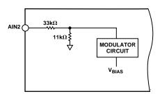
Figure 8. AIN2 Input Impedance
