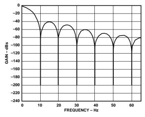
Figure 6. Frequency Response of AD7712 Filter
