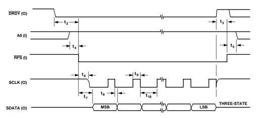
Figure 11. Self-Clocking Mode, Output Data Read Operation
