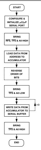
Figure 17. Flowchart for Single Write Operation to the AD7712
