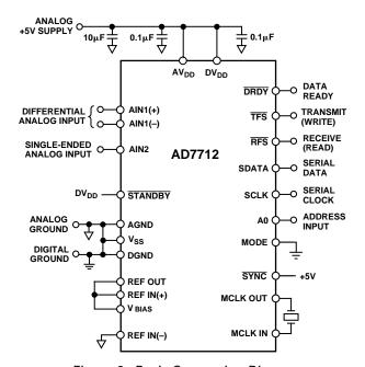
Figure 3. Basic Connection Diagram
