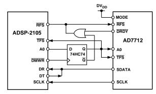
Figure 20. AD7712 to ADSP-2105 Interface
