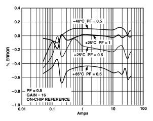
Figure 9. Error as a % of Reading (Gain = 16)
