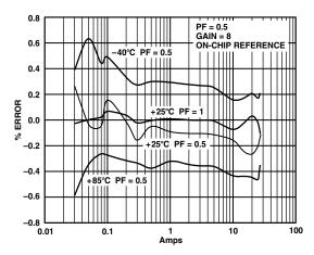
Figure 8. Error as a % of Reading (Gain = 8)
