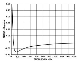
Figure 28. Phase Error Between Channels (0 Hz to 1 kHz)
