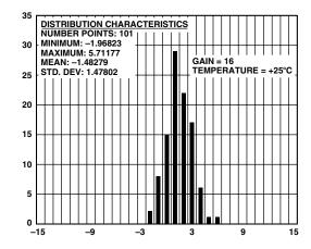
Figure 18. Channel 1 Offset Distribution (Gain = 16)
