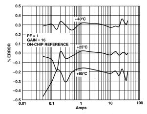
Figure 5. Error as a % of Reading (Gain = 16)
