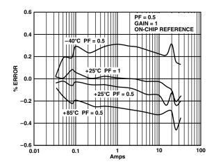
Figure 6. Error as a % of Reading (Gain = 1)
