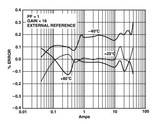
Figure 11. Error as a % of Reading over Temperature with an External Reference (Gain = 16)
