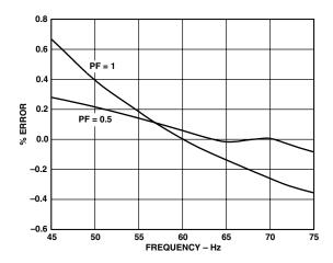
Figure 12. Error as a % of Reading over Frequency
