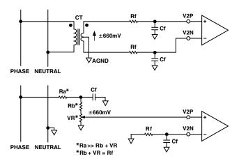
Figure 25. Typical Connections for Channel 2
