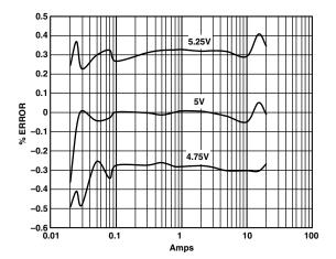
Figure 19. PSR with External Reference (Gain = 16)
