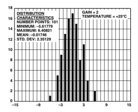
Figure 15. Channel 1 Offset Distribution (Gain = 2)
