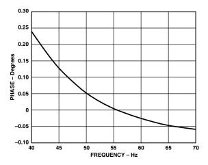
Figure 29. Phase Error Between Channels (40 Hz to 70 Hz)
