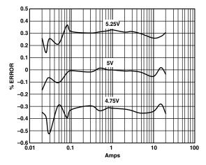
Figure 16. PSR with Internal Reference (Gain = 16)
