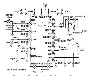
Figure 13. Test Circuit for Performance Curves
