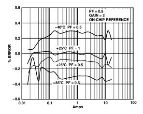
Figure 7. Error as a % of Reading (Gain = 2)
