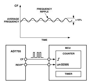
\*REVP MUST BE USED IF THE METER IS BIDIRECTIONAL OR DIRECTION OF ENERGY FLOW IS NEEDED
