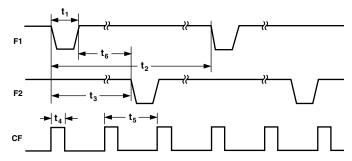
Figure 1. Timing Diagram for Frequency Outputs
