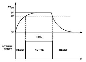
Figure 26. On-Chip Power Supply Monitor
