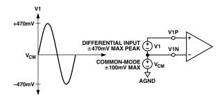
Figure 22. Maximum Signal Levels, Channel 1, Gain = 1
