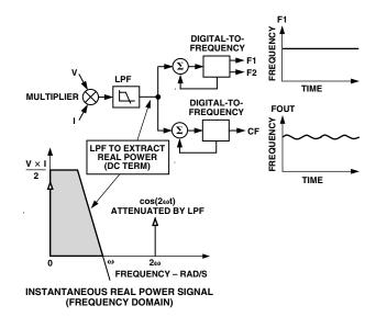
Figure 30. Real Power-to-Frequency Conversion
