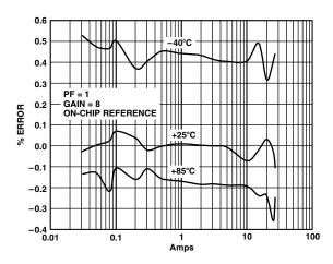
Figure 4. Error as a % of Reading (Gain = 8)
