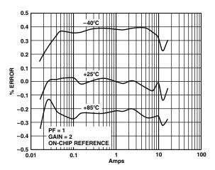
Figure 3. Error as a % of Reading (Gain = 2)
