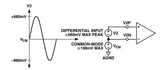
Figure 23. Maximum Signal Levels, Channel 2
