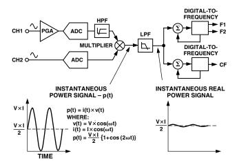
Figure 20. Signal Processing Block Diagram
