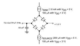
Figure 1. Load Circuit for Timing Characterization
