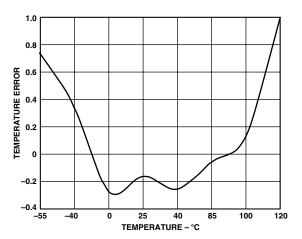
Figure 7. Typical Temperature Error
