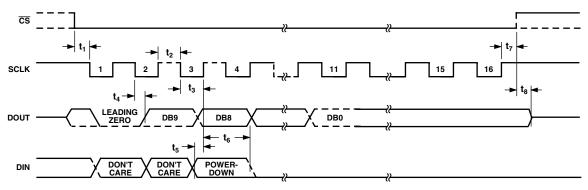
Figure 2. Serial Interface Timing Diagram
