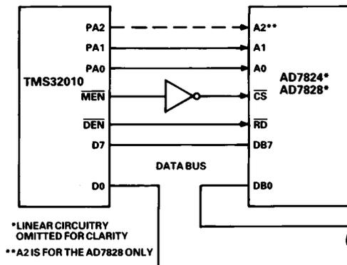
Figure 18. AD7824/AD7828-TMS32010 Interface
