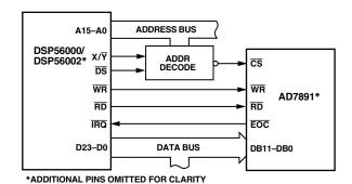
Figure 15. AD7891 to DSP5600x Parallel Interface
