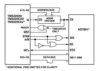
Figure 13. AD7891 to TMS32020/C25/C5x Parallel Interface
