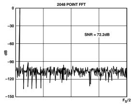
Figure 18. Typical AD7891-1 FFT Plot
