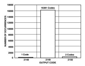
Figure 17. Typical Histogram Plot (AD7891-1)
