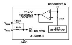
Figure 6. AD7891-2 Analog Input Structure
