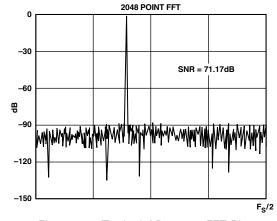
Figure 19. Typical AD7891-2 FFT Plot
