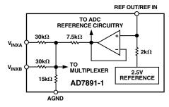
Figure 5. AD7891-1 Analog Input Structure
