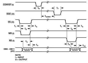
Figure 2. Parallel Mode Timing Diagram
