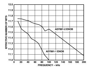
Figure 20. Effective Number of Bits vs. Frequency
