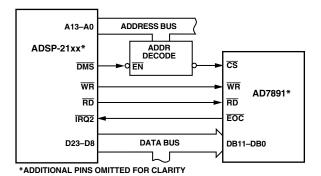
Figure 12. AD7891 to ADSP-21xx Parallel Interface
