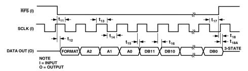
Figure 3. Serial Mode Read Operation
