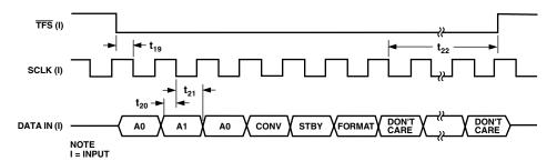
Figure 4. Serial Mode Write Operation
