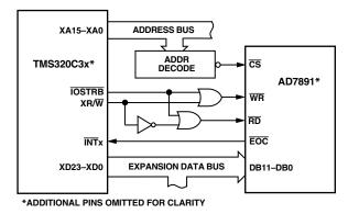
Figure 14. AD7891 to TMS320C30 Parallel Interface
