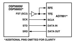
Figure 10. AD7891 to DSP5600x Serial Interface
