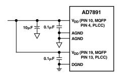
Figure 16. Recommended Decoupling Scheme for the AD7891
