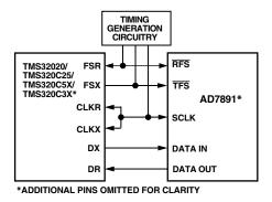
Figure 11. AD7891 to TMSxxx Serial Interface
