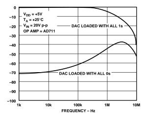
Figure 12. Multiplying Frequency Response vs. Digital Code
