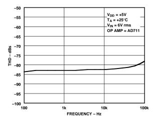
Figure 10. Total Harmonic Distortion vs. Frequency
