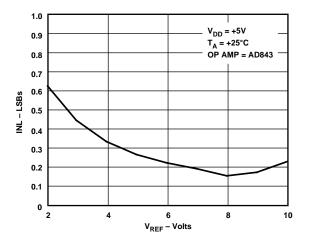
Figure 6. Integral Nonlinearity Error vs.  $V_{REF}$  (Normal Mode)
