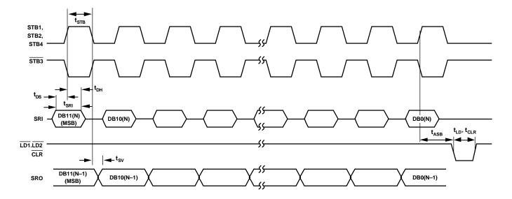
Figure 1. AD7943 Timing Diagram
