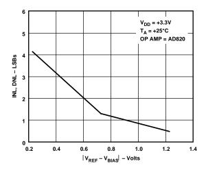
Figure 8. Linearity Error vs. V<sub>REF</sub> (Biased Mode)
