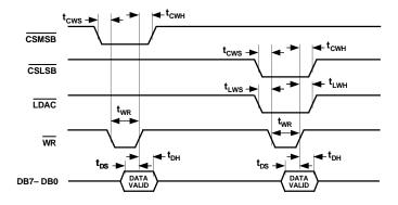
Figure 4. AD7948 Timing Diagram
