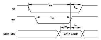
Figure 3. AD7945 Timing Diagram
