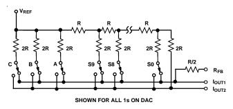
Figure 13. Simplified D/A Circuit Diagram
