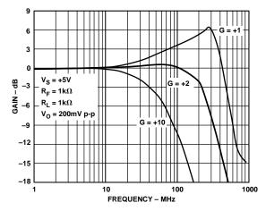
Figure 12. Bandwidth vs. Gain—Single Supply
