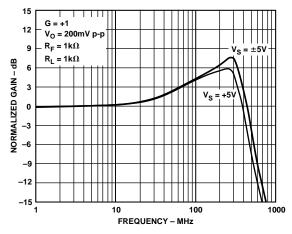
Figure 1. Frequency Response, G = +1,  $V_S = \pm 5$  V and +5 V
