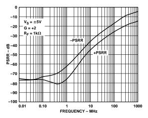
Figure 13. PSRR vs. Frequency
