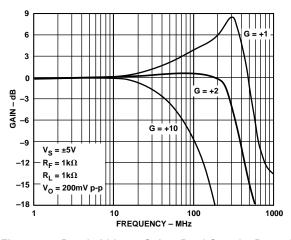
Figure 11. Bandwidth vs. Gain—Dual Supply,  $R_F = 1 \text{ k}\Omega$
