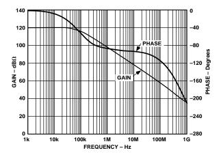
Figure 16. Transimpedance Gain and Phase vs. Frequency
