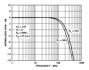
Figure 2. Frequency Response, G = +2,  $V_O = 2 V p-p$
