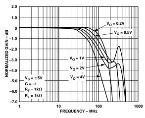
Figure 4. Bandwidth vs. Output Level—Gain of –1, Dual Supply
