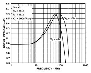
Figure 9. Gain Flatness—Small Signal
