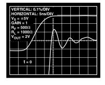
Figure 18. Settling Time
