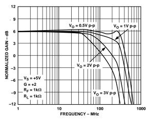
Figure 5. Bandwidth vs. Output Level—Single Supply, G = +2
