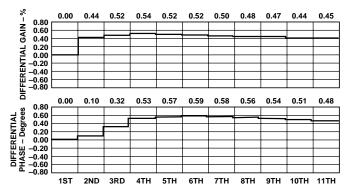
Figure 25. Differential Gain and Phase  $R_F$  = 500,  $\pm 5$  V,  $R_L$  = 50  $\Omega$ , Driving Three Cables, G = +2
