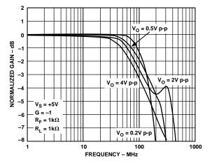
Figure 6. Bandwidth vs. Output Level—Single Supply, Gain of –1
