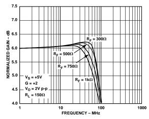
Figure 8. Bandwidth vs. Feedback Resistor—Single Supply
