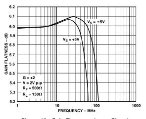
Figure 10. Gain Flatness—Large Signal
