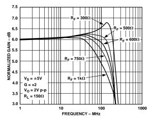
Figure 7. Bandwidth vs. Feedback Resistor—Dual Supply
