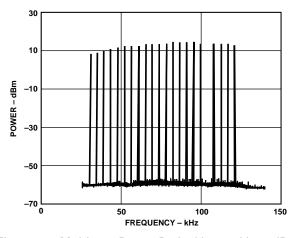
Figure 28. Multitone Power Ratio:  $V_S$  =  $\pm 6$  V, 27 dBm Output Power into 25  $\Omega$
