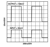
Figure 5. 100 mV Step Response; G = +2,  $V_S$  =  $\pm 2.5$  V or  $\pm 6$  V,  $R_L$  = 100  $\Omega$
