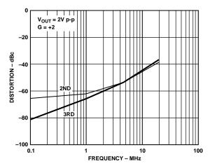
Figure 11. Distortion vs. Frequency;  $V_S = \pm 6 \text{ V}$ ,  $R_L = 25 \Omega$
