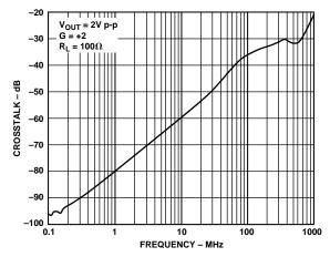
Figure 35. Output Crosstalk vs. Frequency
