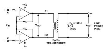
Figure 2. Differential Drive Circuit for xDSL Applications
