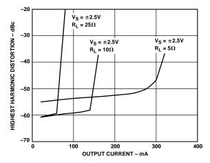
Figure 15. Distortion vs. Output Current;  $V_S = \pm 2.5 \text{ V}$ , f = 1 MHz, G = +2
