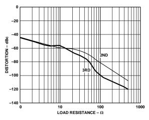
Figure 19. Distortion vs.  $R_L$ ,  $V_S = \pm 2.5$  V, G = +2,  $V_{OUT} = 2$  V p-p, f = 1 MHz
