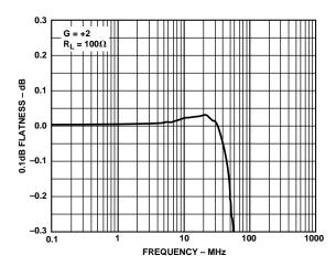
Figure 26. Gain Flatness;  $V_S = \pm 2.5 \text{ V}$
