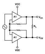
Figure 40. Differential Driver Simplified Circuit Schematic
