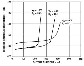
Figure 12. Distortion vs. Output Current;  $V_S = \pm 6 V$ , f = 1 MHz, G = +2
