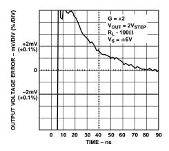
Figure 34. Settling Time;  $V_S = \pm 6.0 \text{ V}$
