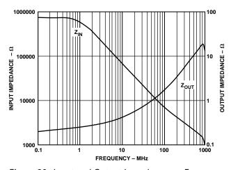
Figure 36. Input and Output Impedance vs. Frequency
