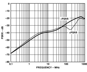
Figure 32. PSRR vs. Frequency;  $V_S = \pm 6 \text{ V or } V_S = \pm 2.5 \text{ V}$
