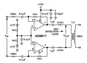
Figure 39. Single +12 V Supply ADSL Remote Terminal Transmitter
