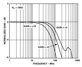
Figure 22. Frequency Response;  $V_S = \pm 6 \ V$
