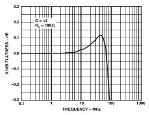
Figure 23. Gain Flatness;  $V_S = \pm 6 V$
