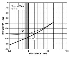
Figure 14. Distortion vs. Frequency;  $V_S = \pm 2.5 \text{ V}$ ,  $R_L = 25 \Omega$
