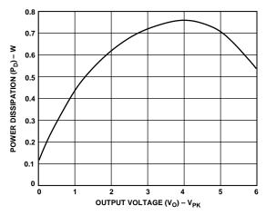
Figure 41. Power Dissipation ( $P_D$ ) vs. Output Voltage ( $V_O$ ),  $R_I = 50 \Omega$
