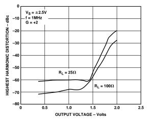
Figure 20. Distortion vs. Output Voltage,  $V_S = \pm 2.5 \text{ V}$ , G = +2, f = 1 MHz
