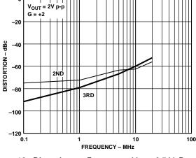
Figure 13. Distortion vs. Frequency;  $V_S = \pm 2.5 \ V, R_L = 100 \ \Omega$
