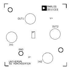
Figure 42. Universal SOIC Noninverter Top Silkscreen
