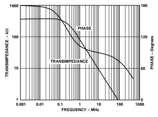
Figure 33. Open-Loop Transimpedance and Phase vs. Frequency
