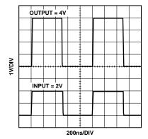
Figure 6. 4 V Step Response; G = +2,  $V_S = \pm 6$  V,  $R_L = 100~\Omega$
