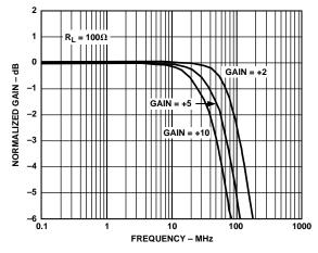
Figure 25. Frequency Response;  $V_S = \pm 2.5 \text{ V}$
