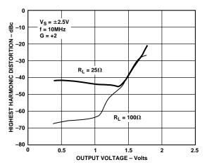
Figure 21. Distortion vs. Output Voltage,  $V_S = \pm 2.5 \text{ V}$ , G = +2, f = 10 MHz
