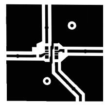
Figure 43. Universal SOIC Noninverter Top
