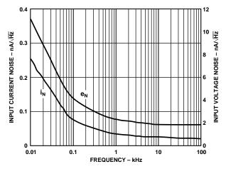
Figure 30. Noise vs. Frequency
