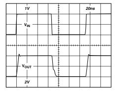
TPC 24. Large Signal Pulse Response, Gain = +2  $(R_{FB} = 750 \,\Omega, \, R_L = 150 \,\Omega, \, V_S = \pm 7.5 \,V)$
