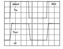
TPC 26. Large Signal Pulse Response, Gain = +10 ( $R_{FB}$  = 400  $\Omega$ ,  $R_L$  = 150  $\Omega$ ,  $V_S$  = ±7.5 V)
