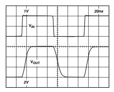
Figure 1. Pulse Response Driving a Large Load Capacitance,  $C_L$  = 300 pF, G = +3,  $R_{FB}$  = 2.32 k $\Omega$ ,  $R_S$  = 10.5  $\Omega$ ,  $R_L$  = 1 k $\Omega$ ,  $V_S$  = ±7.5 V
