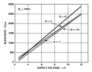
TPC 16. Maximum Slew Rate vs. Supply Voltage
