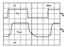
Figure 5. 15% Overload Recovery, Gain = +10  $(R_{FB} = 400 \,\Omega, \, R_L = 1 \, k\Omega, \, V_S = \pm 7.5 \, V)$
