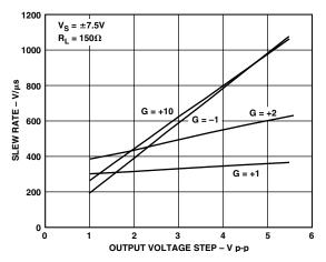
TPC 15. Slew Rate vs. Output Step Size
