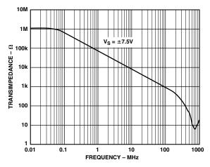
TPC 10. Open-Loop Transimpedance vs. Frequency,  $R_L = 150 \,\Omega$
