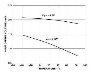
TPC 7. Input Offset Voltage vs. Temperature
