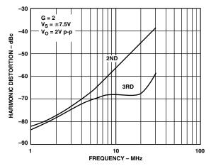
TPC 13. Harmonic Distortion vs. Frequency,  $R_L$  = 150  $\Omega$
