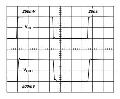
TPC 23. Small Signal Pulse Response, Gain = +2  $(R_{FB} = 750 \,\Omega, \, R_L = 150 \,\Omega, \, V_S = \pm 7.5 \,V)$
