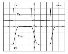
Figure 4. Pulse Response Driving a Large Load Capacitance,  $C_L$  = 300 pF, G = +3,  $R_{FB}$  = 2.32 k $\Omega$ ,  $R_S$  = 10.5  $\Omega$ ,  $R_L$  = 1 k $\Omega$ ,  $V_S$  = ±7.5 V
