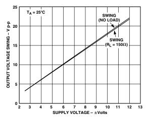
TPC 3. Output Voltage Swing vs. Supply Voltage
