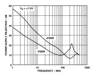
TPC 12. Power Supply Rejection vs. Frequency
