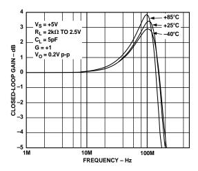
Figure 16. Closed-Loop Frequency Response vs. Temperature
