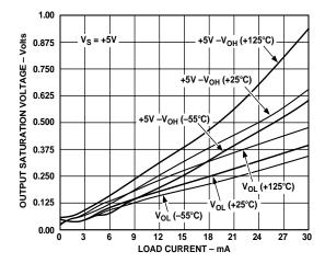
Figure 21. Output Saturation Voltage vs. Load Current
