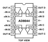
The output voltage swing extends to within 25 mV of each rail, providing the maximum output dynamic range. Additionally, it features gain flatness of 0.1 dB to 12 MHz while offering differential gain and phase error of 0.04% and 0.22° on a single +5 V supply. This makes the AD8044 useful for video electronics such as cameras, video switchers or any high speed portable equipment. The AD8044's low distortion and fast settling make it ideal for active filter applications.
