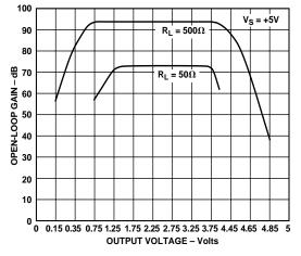
Figure 9. Open-Loop Gain vs. Output Voltage
