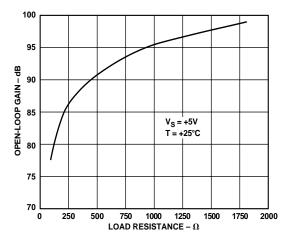
Figure 7. Open-Loop Gain vs. R<sub>L</sub> to +2.5 V
