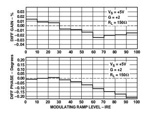
Figure 13. Differential Gain and Phase Errors
