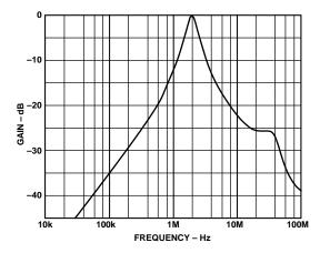
Figure 39. Frequency Response of 2 MHz Bandpass Biquad Filter
