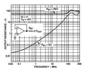
Figure 18. Output Resistance vs. Frequency
