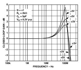
Figure 17. Closed-Loop Frequency Response vs. Supply
