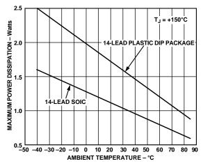
Figure 3. Maximum Power Dissipation vs. Temperature
