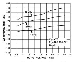
Figure 12. Worst Harmonic vs. Output Voltage
