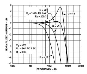
Figure 26. Frequency Response vs. Closed-Loop Gain
