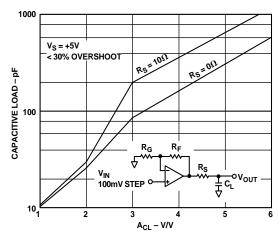
Figure 35. Capacitive Load Drive vs. Closed-Loop Gain
