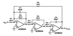
Figure 38. 2 MHz Biquad Bandpass Filter Using AD8044
