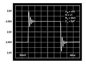
Figure 30. 100 mV Step Response,  $V_S = +5 \text{ V}$ , G = +1
