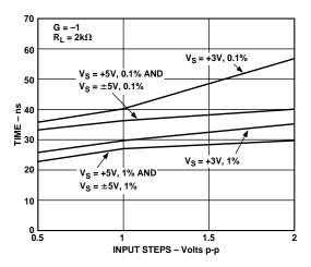
Figure 19. Settling Time vs. Input Step
