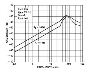
Figure 27. Crosstalk (Output to Output) vs. Frequency
