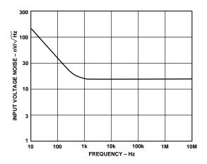
Figure 10. Input Voltage Noise vs. Frequency
