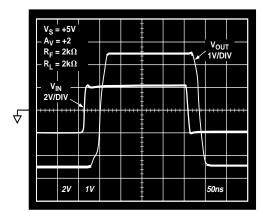
Figure 33. Overdrive Recovery, VS + 5 V, V<sub>IN</sub> = 4 V Step
