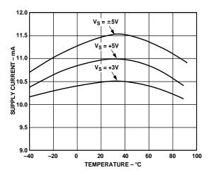
Figure 22. Supply Current vs. Temperature
