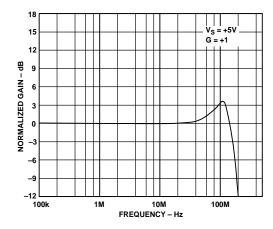
Figure 2. Frequency Response: Gain = +1,  $V_S = +5$  V
