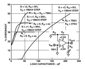
Figure 25. % Overshoot vs. Capacitive Load
