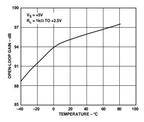
Figure 8. Open-Loop Gain vs. Temperature
