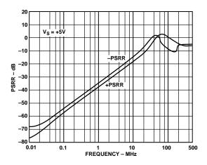
Figure 23. PSRR vs. Frequency
