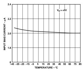
Figure 6. I<sub>B</sub> vs. Temperature
