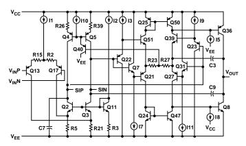
Figure 34. AD8044 Simplified Schematic
