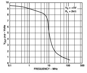
Figure 24. Output Voltage Swing vs. Frequency
