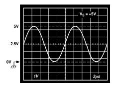
Figure 1. Output Swing: Gain = -1,  $R_L = 2 k\Omega$
