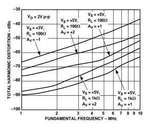
Figure 11. Total Harmonic Distortion
