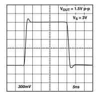
Figure 21. Large Signal Transient Response
