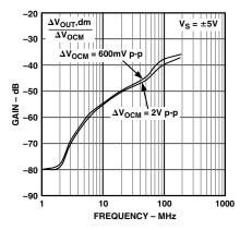
Figure 35. V<sub>OCM</sub> CMRR vs. Frequency
