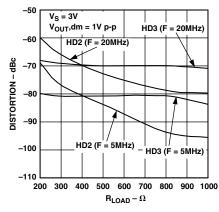
Figure 15. Harmonic Distortion vs.  $R_{LOAD}$
