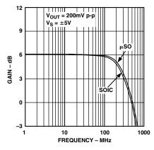
Figure 3. Small Signal Frequency Response
