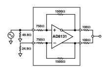
Figure 29. Output Balance Error Test Circuit
