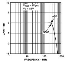
Figure 5. Large Signal Frequency Response
