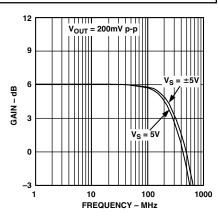
Figure 4. Small Signal Frequency Response
