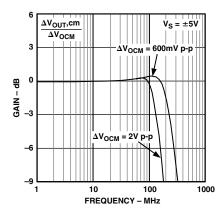
Figure 34.  $V_{OCM}$  Gain Response
