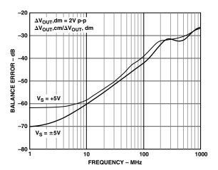
Figure 1. Output Balance Error vs. Frequency
