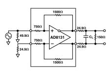
Figure 23. Capacitor Load Drive Test Circuit
