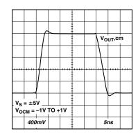
Figure 36. V<sub>OCM</sub> Transient Response
