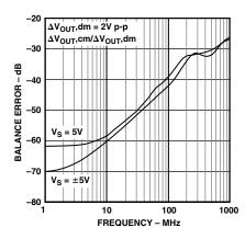
Figure 30. Output Balance Error vs. Frequency
