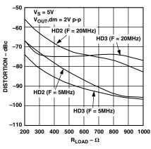
Figure 14. Harmonic Distortion vs.  $R_{LOAD}$
