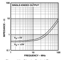
Figure 28. Single-Ended  $Z_{OUT}$  vs. Frequency
