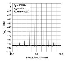
Figure 16. Intermodulation Distortion
