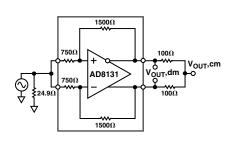
Figure 26. CMRR Test Circuit
