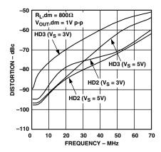
Figure 8. Harmonic Distortion vs. Frequency
