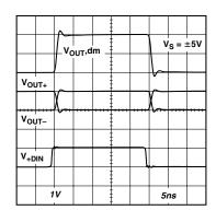
Figure 18. Large Signal Transient Response
