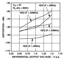
Figure 12. Harmonic Distortion vs. Differential Output Voltage
