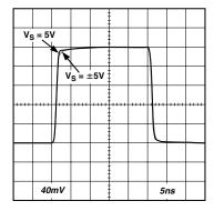
Figure 19. Small Signal Transient Response
