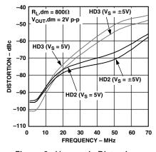
Figure 9. Harmonic Distortion vs. Frequency
