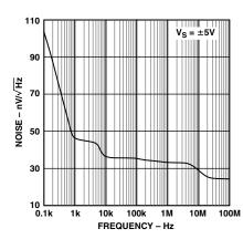
Figure 33. Voltage Noise vs. Frequency
