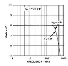
Figure 6. Large Signal Frequency Response
