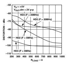
Figure 13. Harmonic Distortion vs.  $R_{LOAD}$
