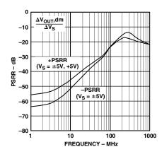
Figure 25. PSRR vs. Frequency
