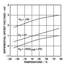
Figure 31. Output Offset Voltage vs. Temperature
