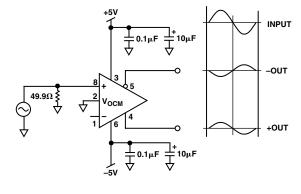
Figure 41. Unity Gain, Single-Ended-to-Differential Amplifier
