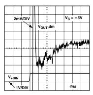
Figure 22. 0.1% Settling Time
