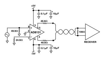
Figure 38. Single-Ended-to-Differential 100  $\Omega$  Line Driver
