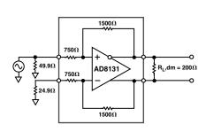
Figure 2. Basic Test Circuit
