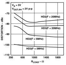
TPC 13. Harmonic Distortion vs.  $R_{LOAD}$
