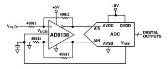
The AD8138 eliminates the need for a transformer with high performance ADCs, preserving the low frequency and dc information. The common-mode level of the differential output is adjustable by a voltage on the  $V_{OCM}$  pin, easily level-shifting the input signals for driving single-supply ADCs. Fast overload recovery preserves sampling accuracy.
