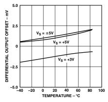
TPC 30. Output Referred Differential Offset Voltage vs. Temperature
