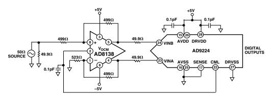
Figure 6. AD8138 Driving an AD9224, a 12-Bit, 40 MSPS A/D Converter
