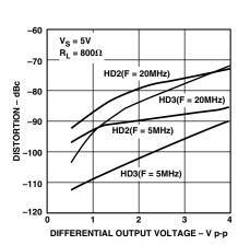
TPC 11. Harmonic Distortion vs. Differential Output Voltage
