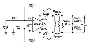
Figure 4. AD8138 Forms a Balanced Transformer Driver
