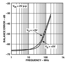
*TPC 27. Output Balance Error vs. Frequency*
