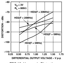
TPC 12. Harmonic Distortion vs. Differential Output Voltage
