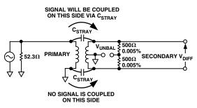
Figure 3. Transformer Single-Ended-to-Differential Converter Is Inherently Imbalanced
