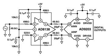
*Figure 7. AD8138 Driving an AD9203, a 10-Bit, 40 MSPS A/D Converter*
