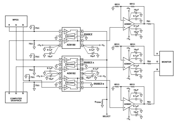
Figure 23. Multiplexing Two Component Video Sources
