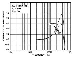
Figure 8. Gain Flatness vs. Frequency
