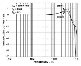
Figure 7. Small Signal Frequency Response
