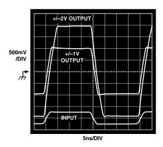
Figure 11. Large Signal Transient Response
