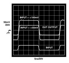
Figure 10. Small Signal Transient Response
