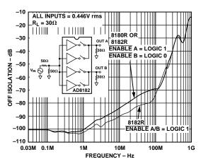
Figure 14. "OFF" Isolation vs. Frequency
