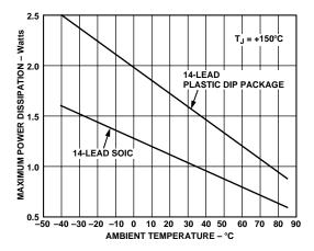
Figure 3. AD8182 Maximum Power Dissipation vs. Temperature
