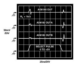
Figure 6. Channel Switching Transient (Glitch)
