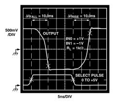
Figure 4. Channel Switching Characteristics
