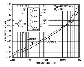
Figure 13. All-Hostile Crosstalk vs. Frequency
