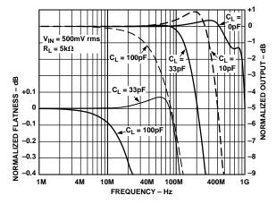
Figure 19. Frequency Response vs. Capacitive Load
