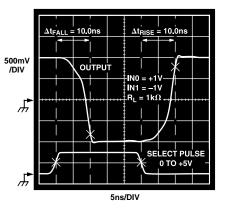
Figure 1. AD8180/AD8182 Switching Characteristics
