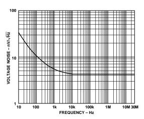
Figure 15. Voltage Noise vs. Frequency
