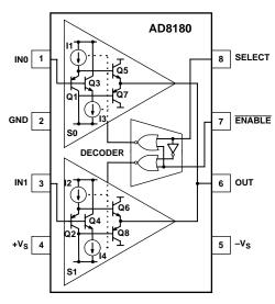
Figure 22. Block Diagram and Simplified Schematic of the AD8180 Multiplexer
