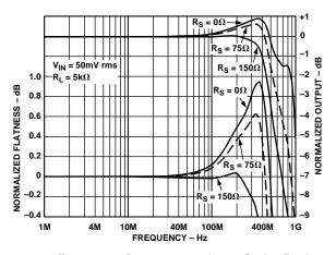
Figure 20. Frequency Response vs. Input Series Resistance
