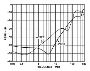
Figure 18. Power Supply Rejection vs. Frequency
