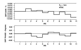
Figure 12. Differential Gain and Phase Error
