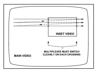
Figure 24. "Picture-in-Picture," Pixel Switching
