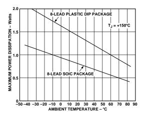
Figure 2. AD8180 Maximum Power Dissipation vs. Temperature
