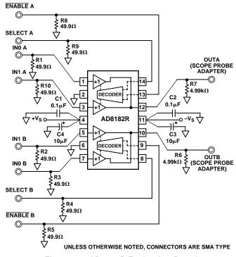
Figure 27. AD8182R Evaluation Board
