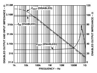
Figure 17. Disabled Output and Input Impedance vs. Frequency
