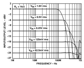
Figure 9. Large Signal Frequency Response
