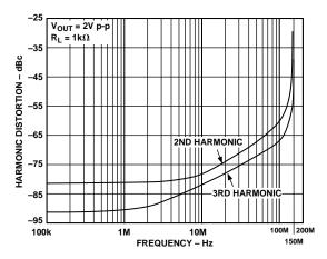
Figure 16. Harmonic Distortion vs. Frequency
