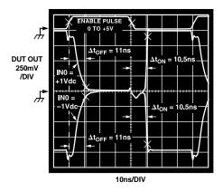
Figure 5. Enable and Disable Switching Characteristics
