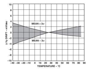
TPC 25. Slope Drift vs. Temperature ( $3\sigma$  to Either Side of Mean of 200 mV/decade)
