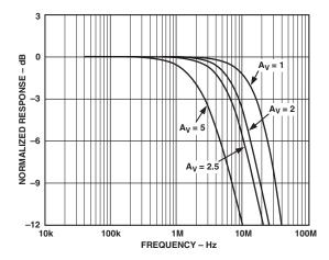
TPC 16. Small Signal AC Response of the Buffer for Various Closed-Loop Gains ( $R_L = 1 \text{ k}\Omega \text{ } C_L < 2 \text{ pF}$ )
