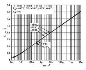
TPC 1.  $V_{LOG}$  vs.  $I_{PD}$  for Multiple Temperatures
