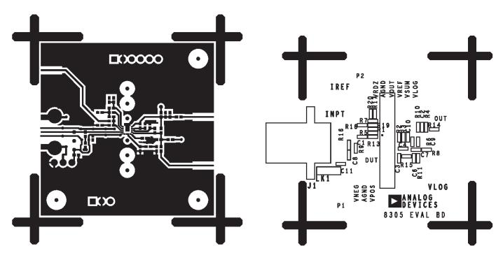
Figure 14. Component Side Layout
