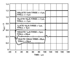
TPC 11. Pulse Response –  $I_{PD}$  to  $V_{OUT}$  (G = 1)
