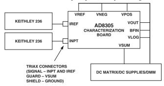
Figure 9. Primary Characterization Setup
