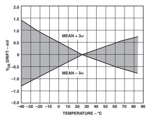
TPC 17. Buffer Input Offset Drift vs. Temperature ( $3\sigma$  to Either Side of Mean)
