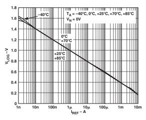
TPC 2. V<sub>LOG</sub> vs. I<sub>REF</sub> for Multiple Temperatures
