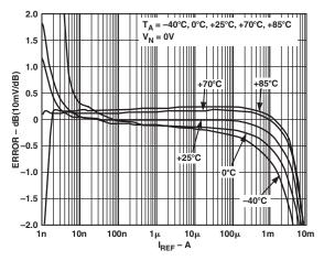
TPC 5. Law Conformance Error vs.  $I_{REF}$  (at  $I_{PD} = 10 \mu A$ ) for Multiple Temperatures, Normalized to 25°C
