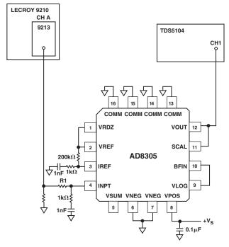
Figure 13. Configuration for Logarithmic Amplifier Pulse Response Measurement
