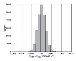
TPC 30. Distribution of Offset Voltage ( $V_{INPT} - V_{SUM}$ ) Sample >22,000
