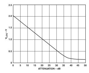
Figure 6. Example of an Absorbance Transfer Function
