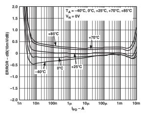
TPC 4. Law Conformance Error vs.  $I_{PD}$  (at  $I_{REF} = 10 \mu A$ ) for Multiple Temperatures, Normalized to 25°C
