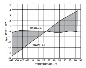
TPC 24.  $V_{\text{INPT}}$  Drift vs. Temperature (3 $\sigma$  to Either Side of Mean)
