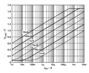
TPC 3.  $V_{LOG}$  vs.  $I_{PD}$  for Multiple Values of  $I_{REF}$ (Decade Steps from 10 nA to 1 mA)
