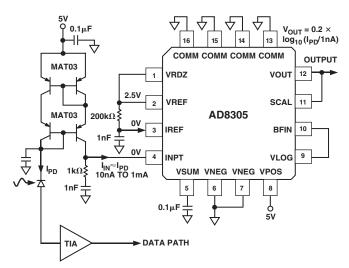
Figure 7. Wilson Current Mirror for Cathode Interfacing
