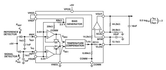
Figure 5. Optical Absorbance Measurement
