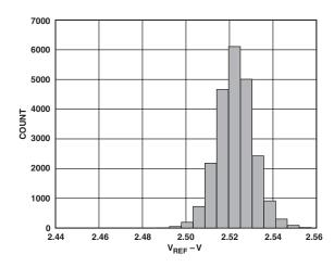
TPC 29. Distribution of  $V_{REF}$  ( $R_L = 100 \text{ k}\Omega$ ) Sample >22,000
