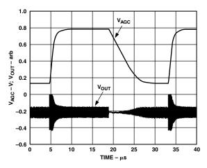
Figure 10. AGC Response to a 32 dB Step in Input Level (f = 50 MHz)
