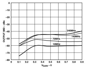
TPC 10. IMD3 vs. Gain ( $V_{OUT} = 1 V p-p Composite$ )
