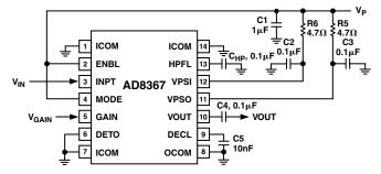
Figure 7. Basic Connections for Voltage-Controlled Gain Mode
