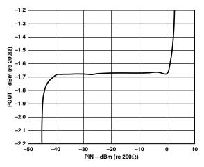
Figure 9. Leveling Accuracy of the AGC Function
