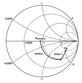
$f_C=140 MHz, Z_{IN}=193.4-j46.3\Omega, Z_{LOAD}=229-j8.8\Omega$   $R_{SOURCE}=50\Omega, R_{LOAD}=50\Omega$
