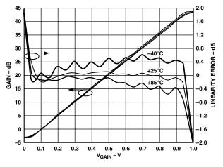
TPC 3. Gain Conformance at 70 MHz for  $T = -40^{\circ}$ C, +25°C, and +85°C.
