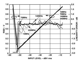
TPC 19. AGC RSSI (Voltage on DETO Pin) vs. Input Power at 10 MHz, 70 MHz, 140 MHz, and 240 MHz
