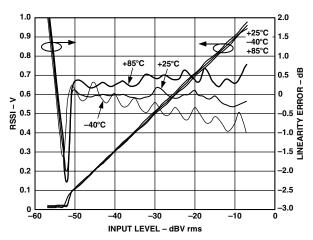
TPC 20. AGC RSSI (Voltage on DETO Pin) vs. Input Power over Temperature at 70 MHz
