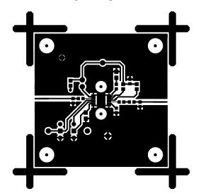
Figure 17. Layout of Component Side
