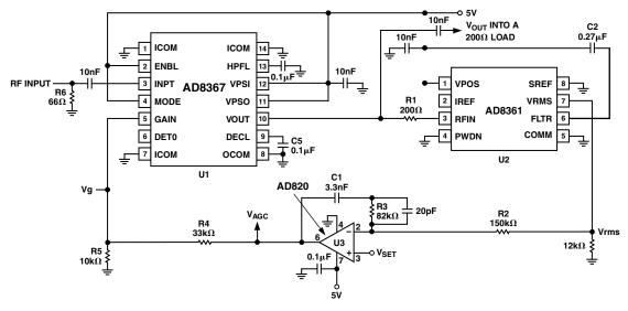
Figure 12. Example of Using an External Detector to Form an AGC Loop
