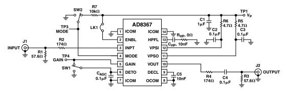
Figure 16. Evaluation Board Schematic
