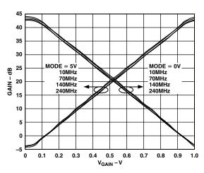
TPC 2. Gain vs.  $V_{GAIN}$  (Mode LO and Mode HI)
