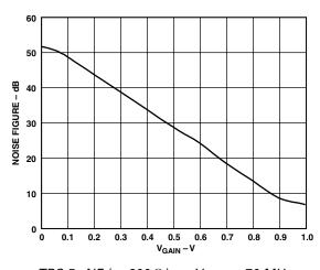
TPC 5. NF (re 200  $\Omega$ ) vs.  $V_{GAIN}$  at 70 MHz
