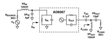
Figure 6. Reactive Matching Example for f = 140 MHz
