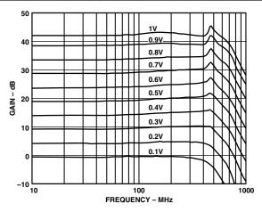
TPC 1. Gain vs. Frequency for Values of  $V_{GAIN}$
