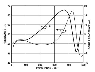
TPC 15. Output Resistance and Series Reactance vs. Frequency at  $V_{GAIN} = 500 \text{ mV}$
