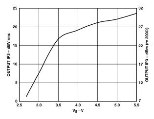
TPC 12. Output Third Order Intercept vs. Supply Voltage at 70 MHz,  $V_{GAIN} = 500 \text{ mV}$
