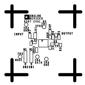
Figure 18. Silkscreen of Component Side
