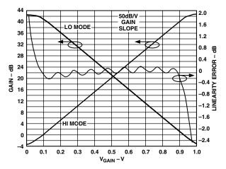
Figure 2. The gain function can be either an increasing or decreasing function of  $V_{\rm GAIN}$  depending on the MODE pin.
