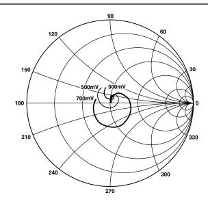
TPC 16. Output Reflection Coefficient vs. Frequency from 10 MHz to 500 MHz for Multiple Values of  $V_{\rm GAIN}$
