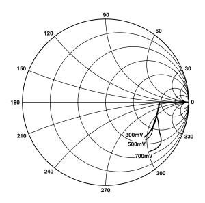
TPC 14. Input Reflection Coefficient vs. Frequency from 10 MHz to 500 MHz for Multiple Values of  $V_{\rm GAIN}$
