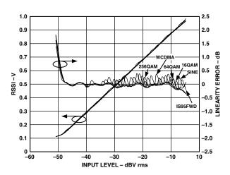
TPC 21. AGC RSSI (Voltage on DETO Pin) vs. Input Power for Various Modulation Schemes
