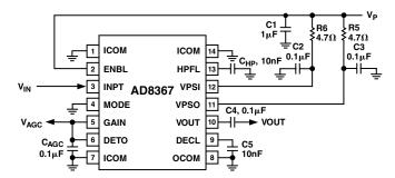
Figure 8. Basic Connections for AGC Operation
