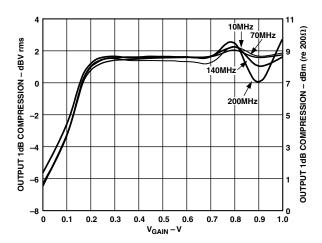
TPC 8. Output P1dB vs. V<sub>GAIN</sub>
