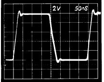
Figure 20b. Noninverting Large Signal Pulse Response
