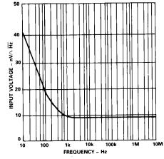
Figure 17. Input Voltage vs. Frequency
