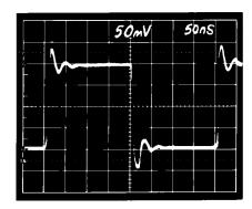
Figure 19c. Inverter Small Signal Pulse Response
