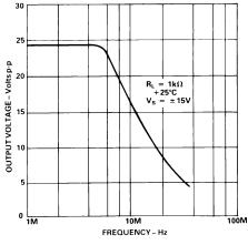
Figure 14. Large Signal Frequency Response
