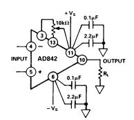
Figure 21. Offset Nulling (DIP Pinout)
