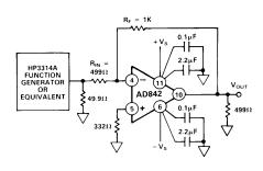
Figure 19a. Inverting Amplifier Configuration (DIP Pinout)
