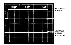
Figure 24. AD842 Settling Demonstrating No Settling Tails
