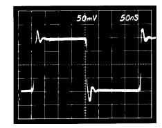
Figure 20c. Noninverting Signal Pulse Response
