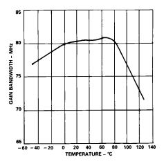
*Figure 9. Gain Bandwidth Product vs. Temperature*
