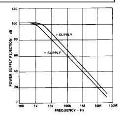
Figure 12. Power Supply Rejection vs. Frequency
