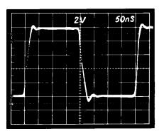
Figure 19b. Inverter Large Signal Pulse Response
