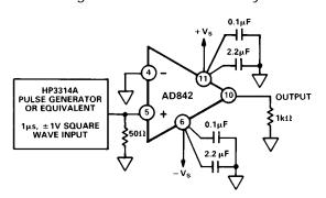
Figure 27. Overdrive Recovery Test Circuit
