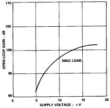
Figure 11. Open-Loop Gain vs. Supply Voltage
