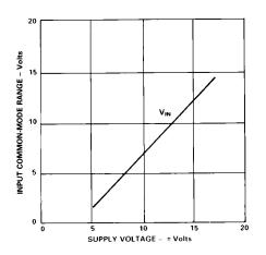
Figure 1. Input Common-Mode Range vs. Supply Voltage
