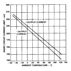
*Figure 8. Short-Circuit Current Limit vs. Temperature*
