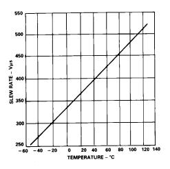
*Figure 18. Slew Rate vs. Temperature*
