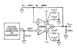
Figure 20a. Noninverting Amplifier Configuration (DIP Pinout)
