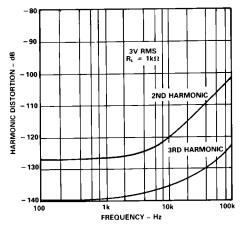
*Figure 16. Harmonic Distortion vs. Frequency*
