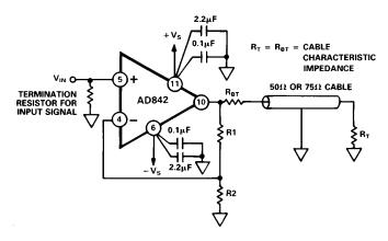
Figure 25. Line Driver Configuration
