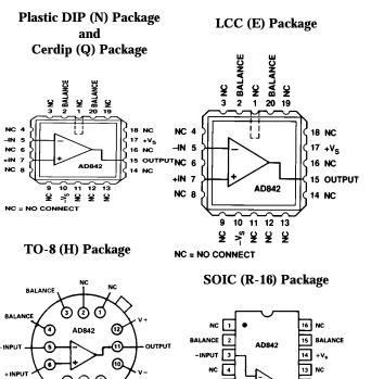
5 12 OUTPUT 11 NC NC 6 7 10 NC -Vs TOP VIEV 8 TOP VIEW 9 NC NOTE: CAN TIED TO V + NC = NO CONNECT NC NC = NO CONNECT AD842 is also appropriate for other applications such as high speed DAC and ADC buffer amplifiers and other wide bandwidth circuitry.
