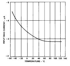
*Figure 5. Input Bias Current vs. Temperature*
