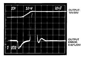
Figure 22. AD842 0.01% Settling Time
