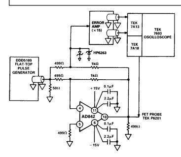
Figure 23. Settling Time Test Circuit
