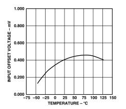
Figure 1. Input Offset Voltage vs. Temperature
