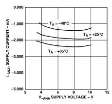
Figure 9. I\_ANA: Analog Supply Current/Comparator vs. Supply Voltage
