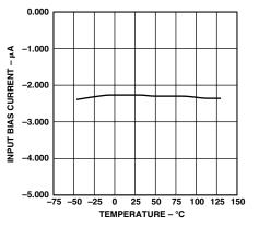
*Figure 2. Input Bias Current vs. Temperature*
