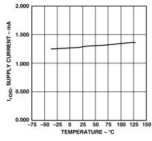
*Figure 13. I*<sub>+DIG</sub>: *Digital Supply Current/ Comparator vs. Temperature*
