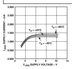
Figure 10. I<sub>+DIG</sub>: Digital Supply Current/Comparator vs. Supply Voltage
