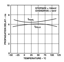
Figure 5. Propagation Delay, t<sub>PDHL</sub>/ t<sub>PDLH</sub> vs. Temperature
