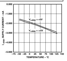
*Figure 12. I*<sub>-ANA</sub>: Analog Supply Current/Comparator vs. Temperature
