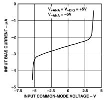
Figure 3. Input Bias Current vs. Input Common-Mode Voltage
