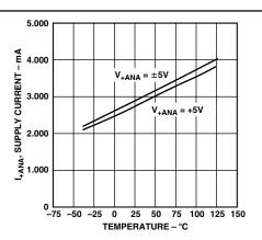
Figure 11. I<sub>+ANA</sub>: Analog Supply Current/Comparator vs. Temperature
