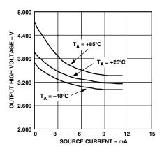
Figure 6. Output High Voltage, V<sub>OH</sub> vs. Source Current
