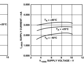
Figure 8. I<sub>+ANA</sub>: Analog Supply Current/Comparator vs. Supply Voltage
