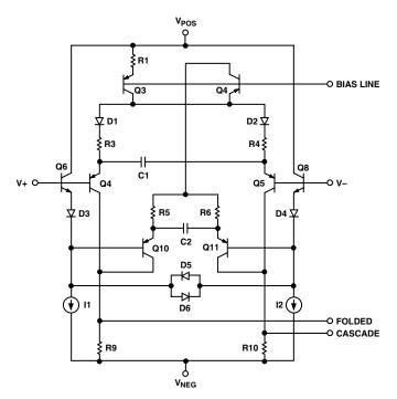
Figure 1. AD856x Equivalent Input Circuit
