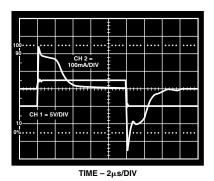
Figure 6. Scope Photo of the  $V_{\rm COM}$  Instantaneous Peak Current
