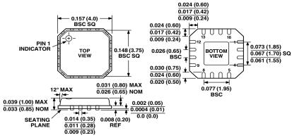
CONTROLLING DIMENSIONS ARE IN MILLIMETERS
