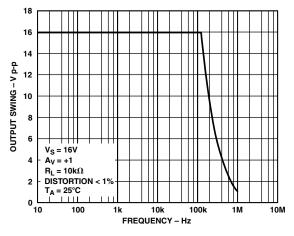
TPC 8. Closed-Loop Output Swing vs. Frequency
