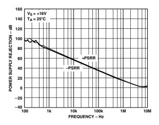
TPC 16. Power Supply Rejection Ratio vs. Frequency
