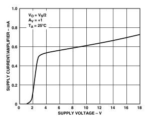
TPC 5. Supply Current/Amplifier vs. Supply Voltage
