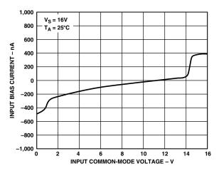
Figure 2. AD856x Input Bias Current vs. Common-Mode Voltage
