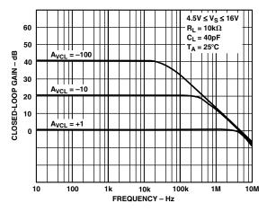
TPC 9. Closed-Loop Gain vs. Frequency
