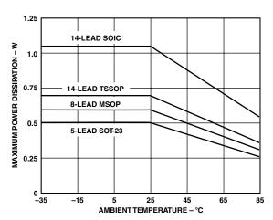
Figure 3. Maximum Power Dissipation vs. Temperature for 5-, 8-, and 14-Lead Packages
