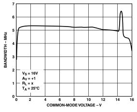
TPC 22. Frequency vs. Common-Mode Voltage ( $V_S = 16 \text{ V}$ )
