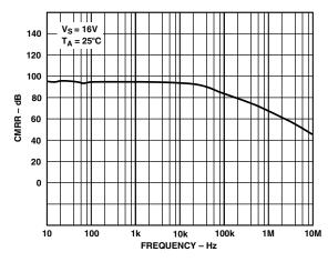
TPC 15. Common-Mode Rejection Ratio vs. Frequency
