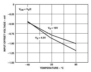
TPC 1. Input Offset Voltage vs. Temperature
