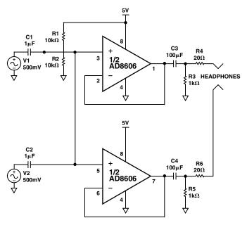
Figure 9. Single-Supply Headphone/Speaker Amplifier
