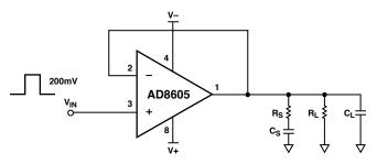
Figure 7. Snubber Network Configuration
