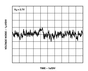
TPC 34. 0.1 Hz to 10 Hz Input Voltage Noise
