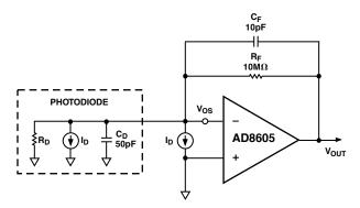
Figure 8. Equivalent Circuit for Photodiode Preamp
