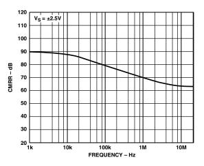
TPC 12. Common-Mode Rejection Ratio vs. Frequency
