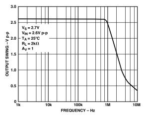
TPC 31. Closed-Loop Output Voltage Swing vs. Frequency
