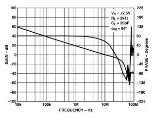
TPC 9. Open-Loop Gain and Phase vs. Frequency
