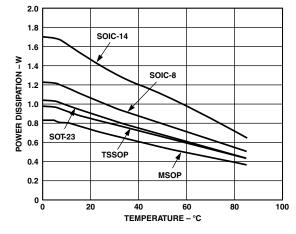
Figure 2. Maximum Power Dissipation vs. Temperature
