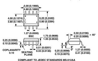
COMPLIANT TO JEDEC STANDARDS MS-012AA CONTROLLING DIMENSIONS ARE IN MILLIMETERS; INCH DIMENSIONS (IN PARENTHESES) ARE ROUNDED-OFF MILLIMETER EQUIVALENTS FOR REFERENCE ONLY AND ARE NOT APPROPRIATE FOR USE IN DESIGN
