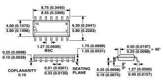
COMPLIANT TO JEDEC STANDARDS MS-012AB CONTROLLING DIMENSIONS ARE IN MILLIMETERS; INCH DIMENSIONS (IN PARENTHESES) ARE ROUNDED-OFF MILLIMETER EQUIVALENTS FOR REFERENCE ONLY AND ARE NOT APPROPRIATE FOR USE IN DESIGN
