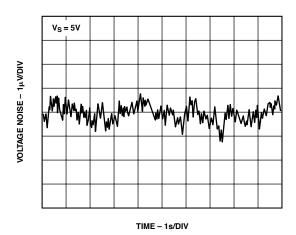
TPC 17. 0.1 Hz to 10 Hz Input Voltage Noise
