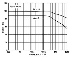
Figure 10. Difference Amplifier CMRR vs. Frequency
