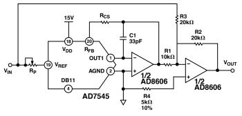
Figure 12. Bipolar Operation
