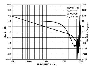
TPC 30. Open-Loop Gain and Phase vs. Frequency
