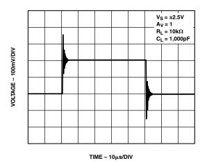
Figure 5. Capacitive Load Drive without Snubber
