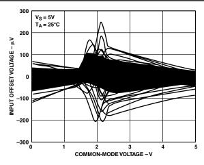
TPC 4. Input Offset Voltage vs. Common-Mode Voltage (200 Units, 5 Wafer Lots, Including Process Skews)
