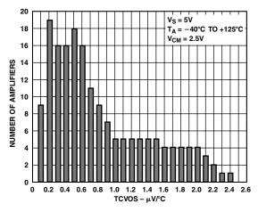
TPC 3. AD8605/AD8606 Input Offset Voltage Drift Distribution
