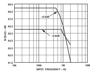
Figure 2. AD871 S/(N+D) vs. Input Frequency
