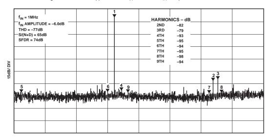
Figure 5. AD871 Typical FFT,  $f_{IN} = 1$  MHz,  $f_{IN}$  Amplitude = -6 dB
