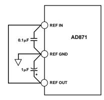
Figure 22. Typical Reference Decoupling Connection
