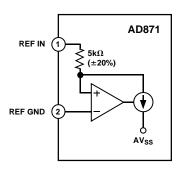
Figure 19. Equivalent Reference Input Circuit
