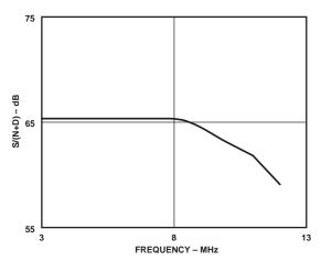
Figure 27. Typical S/(N+D) vs. Clock Frequency  $f_{\rm IN} = 1$  MHz, Full-Scale Input
