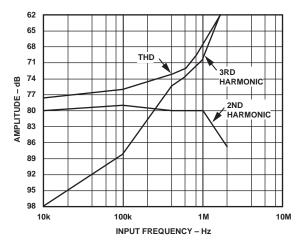
Figure 3. AD871 Distortion vs. Input Frequency, Full-Scale Input
