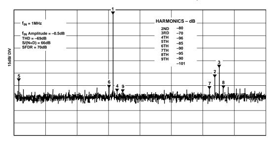
Figure 4. AD871 Typical FFT,  $f_{\rm IN}=1$  MHz,  $f_{\rm IN}$  Amplitude = -0.5 dB
