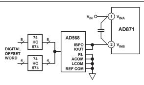
Figure 32. Offset Correction Using the AD568
