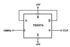
Figure 26. Divide-by-Two Clock Circuit
