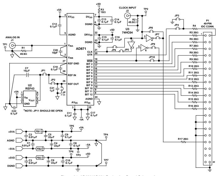
Figure 34. AD872/AD871 Evaluation Board Schematic
