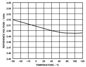
Figure 23. Reference Output Voltage vs. Temperature
