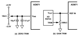
Figure 31. Zero and Gain Error Trims
