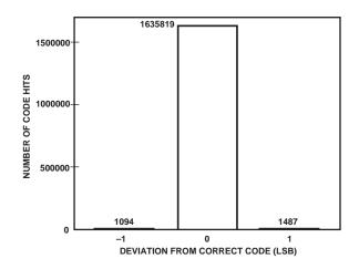
Figure 9. AD871 Code Probability at a Transition
