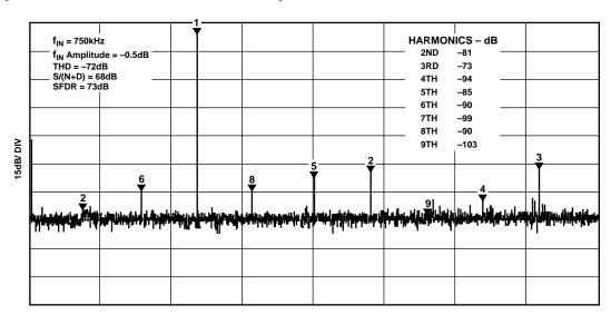
Figure 6. AD871 Typical FFT,  $f_{IN} = 750 \text{ kHz}$
