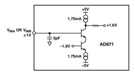
Figure 10. AD871 Equivalent Analog Input Circuit
