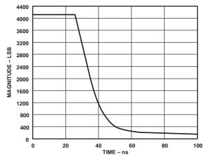
Figure 17. Typical AD871 Settling Time
