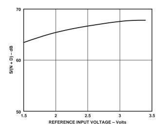
Figure 20. S/(N+D) vs. Reference Input Voltage,  $f_{IN} = 1$  MHz, FS = 5 MHz
