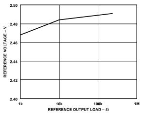
Figure 24. Reference Output Voltage vs. Output Load
