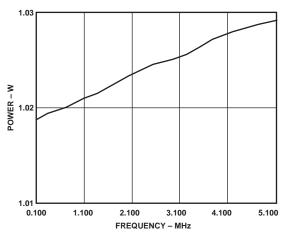
Figure 28. Typical Power Dissipation vs. Clock Frequency
