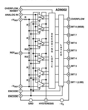
bit to indicate overrange inputs. This overflow output can be disabled with the overflow inhibit pin.
