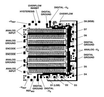
Figure 4. Die Layout and Mechanical Information
