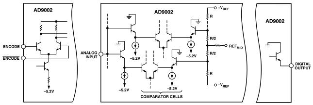
Figure 2. Input/Output Circuits
