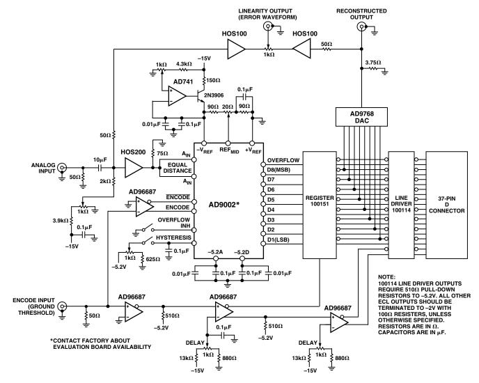
Figure 6. AD9002 Evaluation Circuit
