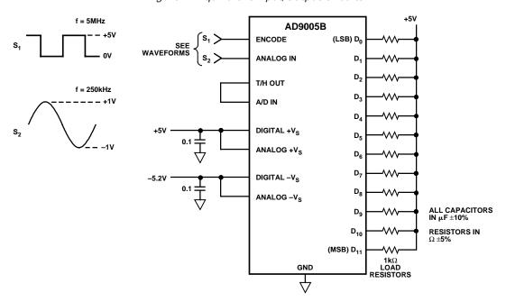
Figure 3. Burn-In Circuit
