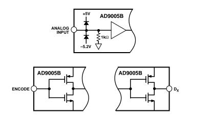
Figure 2. Equivalent Input/Output Circuits
