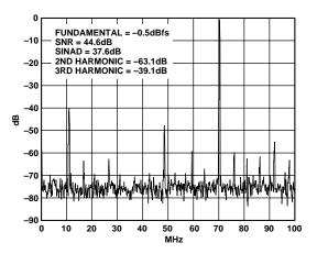
Figure 26. Spectrum:  $f_S = 200 \text{ MSPS}$ ,  $f_{IN} = 70.1 \text{ MHz}$
