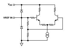
Figure 4. Equivalent Reference Input Circuit
