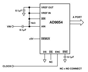
Figure 35. Single Port Mode—AC-Coupled Input—Single-Ended Encode
