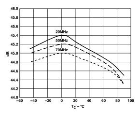
Figure 13. SNR vs. Temperature,  $f_S = 200$  MSPS
