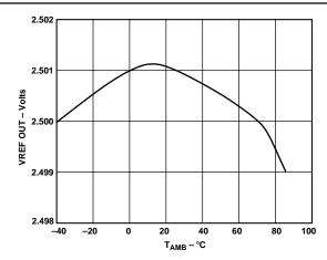
Figure 33. Reference Voltage vs. Temperature
