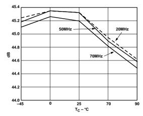
Figure 12. SNR vs. Temperature, f<sub>S</sub> = 135 MSPS
