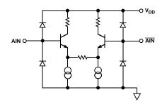
Figure 3. Equivalent Analog Input Circuit
