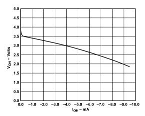
Figure 28. Output Voltage HIGH vs. Output Current
