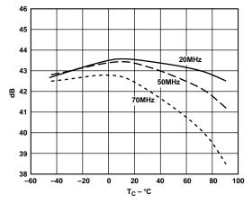
Figure 17. SINAD vs. Temperature:  $f_S = 200 \text{ MSPS}$
