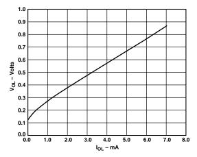
Figure 29. Output Voltage LOW vs. Output Current
