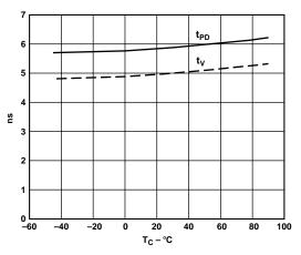
Figure 30. Output Delay vs. Temperature
