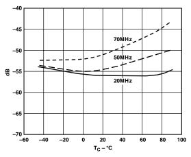
Figure 23. 3rd Harmonic vs. Temperature:  $f_s = 200 \text{ MSPS}$
