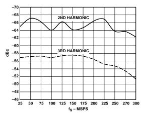
Figure 18. Harmonic Distortion vs.  $f_{S}$ :  $f_{IN} = 19.7 \text{ MHz}$
