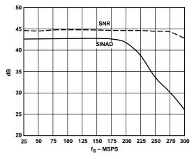
Figure 11. SNR vs. f<sub>S</sub>: f<sub>IN</sub> = 70.1 MHz
