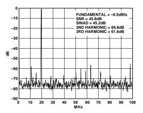
Figure 25. Spectrum:  $f_S = 200 \text{ MSPS}$ ,  $f_{IN} = 19.7 \text{ MHz}$
