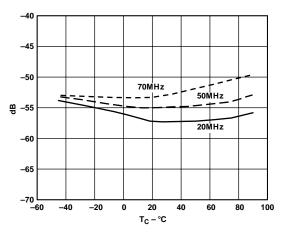
Figure 22. 3rd Harmonic vs. Temperature:  $f_S = 135$  MSPS
