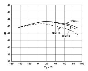
Figure 16. SINAD vs. Temperature:  $f_S = 135$  MSPS
