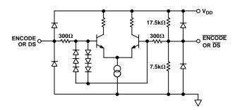
Figure 5. Equivalent ENCODE and Data Select Input Circuit
