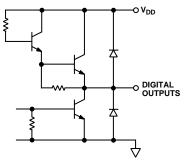
Figure 7. Equivalent Digital Output Circuit
