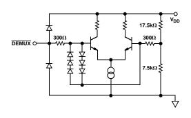
Figure 6. Equivalent DEMUX Input Circuit
