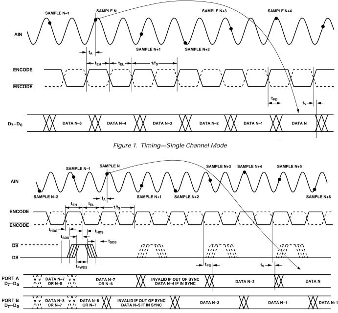
Figure 2. Timing—Dual Channel Mode
