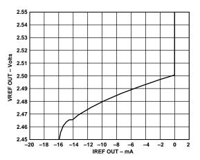
Figure 31. Reference Voltage vs. Reference Load
