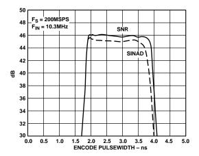
Figure 15. SNR vs. Clock Pulsewidth,  $(t_{PWH})$ :  $f_S = 200 \text{ MSPS}$
