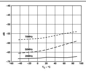
Figure 21. 2nd Harmonic vs. Temperature:  $f_{S} = 200 \text{ MSPS}$
