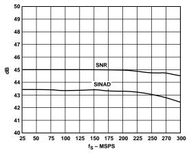
Figure 10. SNR vs.  $f_{S}$ :  $f_{IN} = 19.7 \text{ MHz}$
