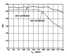
Figure 19. Harmonic Distortion vs.  $f_{S}$ :  $f_{IN}$  = 70.1 MHz
