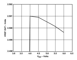
Figure 32. Reference Voltage vs. Power Supply Voltage
