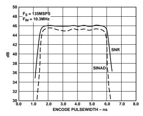
Figure 14. SNR vs. Clock Pulsewidth,  $(t_{PWH})$ :  $f_S = 135$  MSPS
