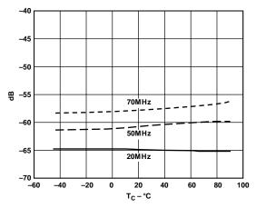
Figure 20. 2nd Harmonic vs. Temperature:  $f_S = 135$  MSPS
