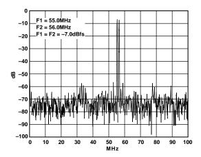
Figure 27. Two Tone Intermodulation Distortion
