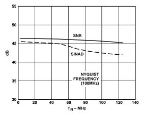
Figure 9. SNR vs.  $f_{IN}$ :  $f_S = 200 \text{ MSPS}$
