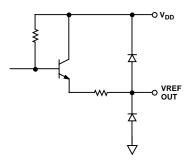
Figure 8. Equivalent Reference Output Circuit
