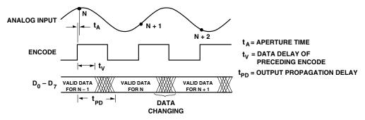
Figure 4. AD9058 Timing Diagram
