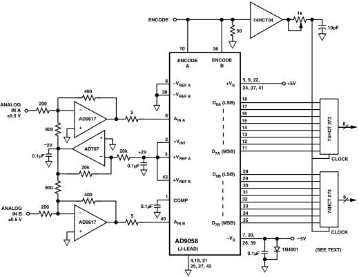
Figure 2. AD9058 Using Internal +2 V Voltage Reference
