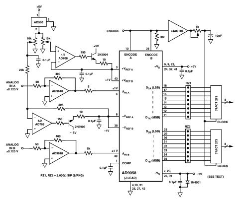
Figure 3. AD9058 Using External Voltage References
