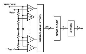
Figure 1. AD9058 Comparator Block Diagram
