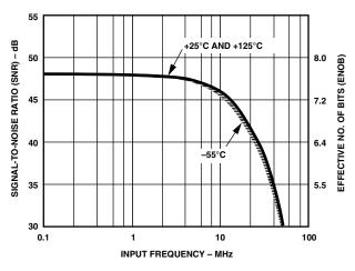
Figure 7. AD9058 Dynamic Performance vs. Analog Input Frequency
