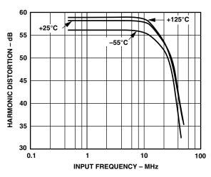
Figure 6. Harmonic Distortion vs. Analog Input Frequency
