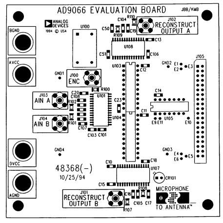
Figure 10. Evaluation Board–Mechanical Layout
