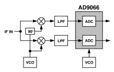
Figure 7. Simplified Block Diagram
