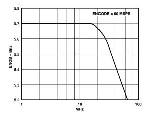
Figure 1. ENOB vs. Analog Input Frequency
