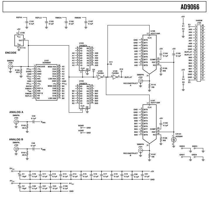
Figure 9. Customer Evaluation Board Schematic
