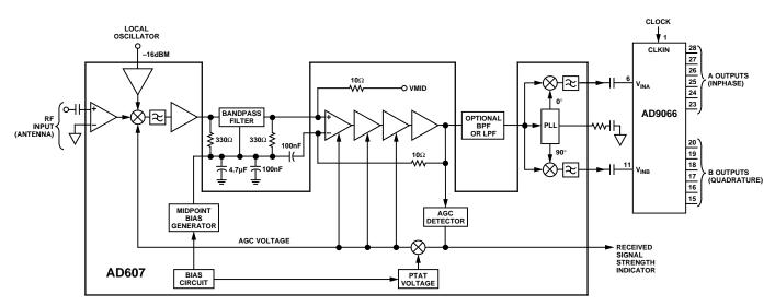
Figure 8. Digitizer with AD607 Receiver Circuit
