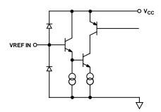
Figure 3. Equivalent Reference Input Circuit
