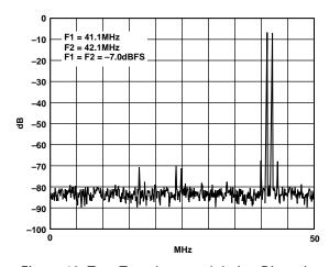
Figure 10. Two-Tone Intermodulation Distortion
