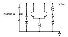
Figure 4. Equivalent Encode Input Circuit
