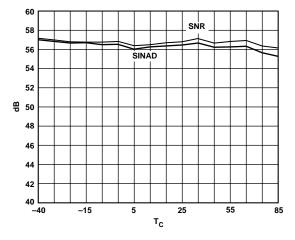
Figure 14. Single-Ended SNR vs.  $T_C$ :  $f_{IN} = 10.3 \text{ MHz}$
