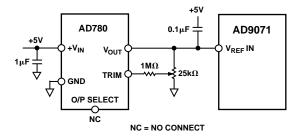
Figure 20. Using the AD780 Voltage Reference
