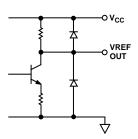
Figure 6. Equivalent Reference Output Circuit
