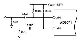
Figure 19. Single-Ended Analog Input Configuration
