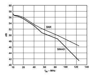
Figure 11. SINAD/SNR vs.  $f_{IN}$ :  $F_S = 100$  MSPS
