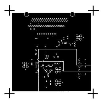
Figure 25. Printed Circuit Board "Split" Power Layer
