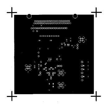
Figure 24. Printed Circuit Board Ground Layer
