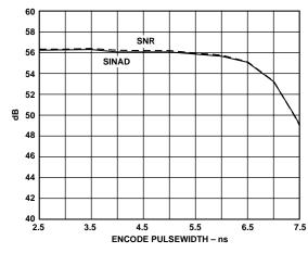
Figure 15. SNR vs. Clock Pulsewidth ( $t_{EH}$ ):  $f_{IN} = 10.3 \text{ MHz}$
