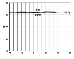
Figure 13. Differential SNR vs.  $T_C$ :  $f_{IN} = 10.3 \text{ MHz}$
