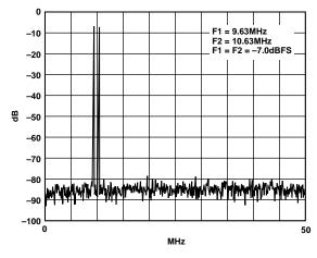
Figure 9. Two-Tone Intermodulation Distortion
