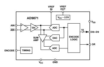
interfacing with 3.3 V or 5 V logic. An out-of-range output (OR) is available that indicates a conversion result is outside the operating range. The output data are held at saturation levels during an out-of-range condition.
