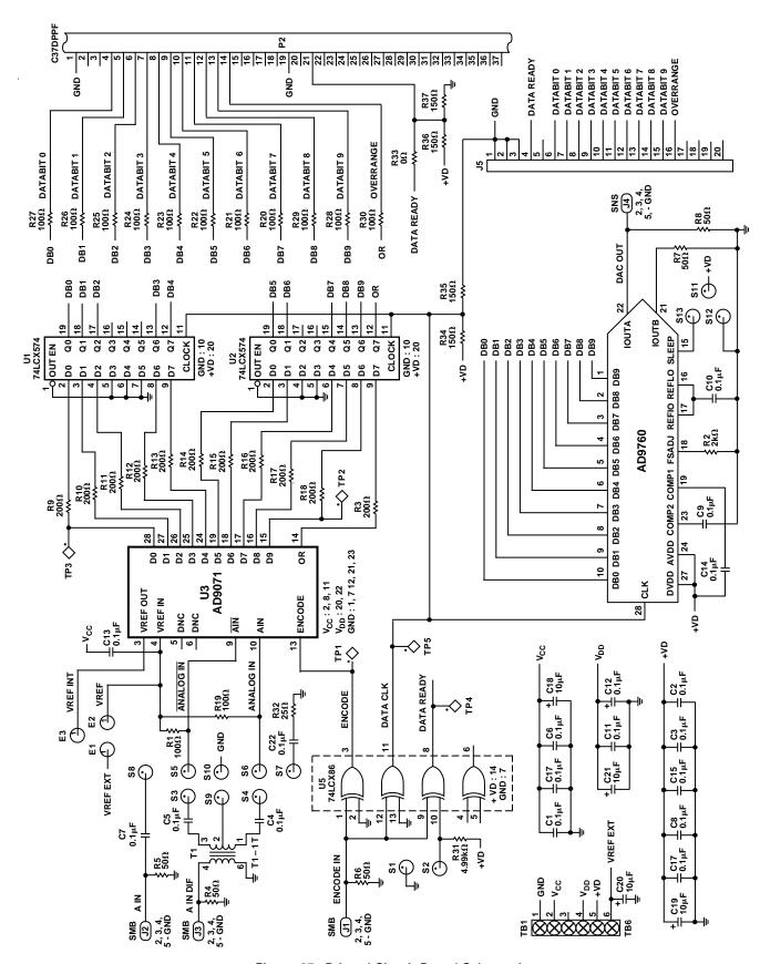
Figure 27. Printed Circuit Board Schematic
