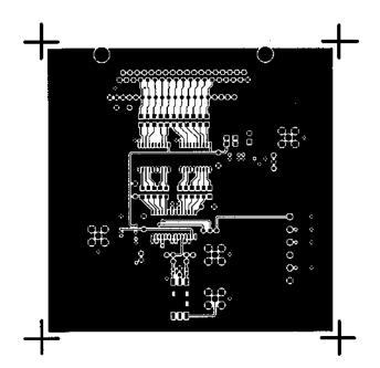
Figure 23. Printed Circuit Board Top Side Copper
