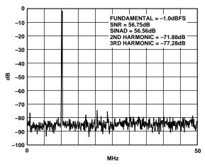
Figure 7. Spectrum:  $F_S = 100$  MSPS,  $f_{IN} = 10.3$  MHz
