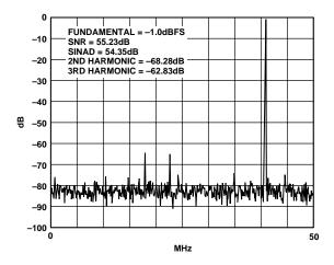
Figure 8. Spectrum:  $F_S = 100$  MSPS,  $f_{IN} = 41$  MHz
