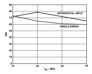
Figure 17. Second Harmonic Performance: Single-Ended vs. Differential Input
