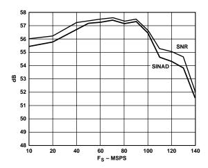
Figure 12. SINAD/SNR vs.  $F_S$ :  $f_{IN} = 10.3 \text{ MHz}$
