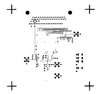
Figure 26. Printed Circuit Board Bottom Side Copper
