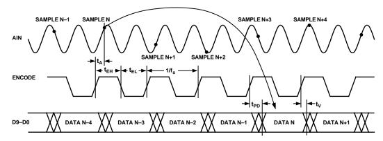
Figure 1. Timing Diagram
