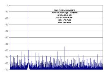
Fig 6 Measured FFT Performance Ain=10.3MHz at 105Msps
