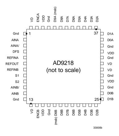
Figure 1. Pin Configuration
