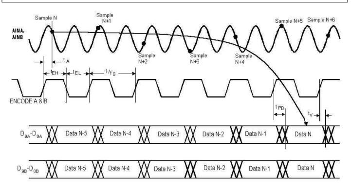
Figure 2. . Normal Operation, Same Clock (S1 =1, S2 = 0) Channel Timing
