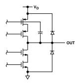
Figure 6. Equivalent Reference Output Circuit
