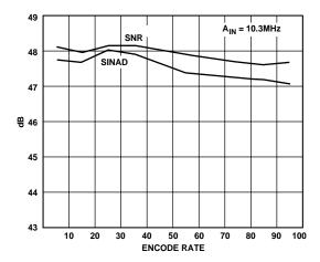
Figure 13. SINAD/SNR vs. Encode Rate
