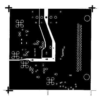
Figure 23. Printed Circuit Board "Split" Power Layer
