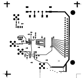
Figure 22. Printed Circuit Board Top Side Copper
