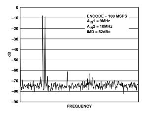
Figure 11. Two-Tone Intermodulation Distortion
