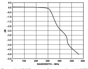
Figure 15. ADC Frequency Response:  $f_S = 100 \text{ MSPS}$
