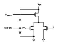
Figure 3. Equivalent Reference Input Circuit
