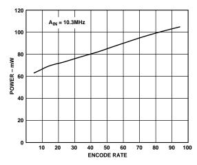
Figure 16. Analog Power Dissipation vs. Encode Rate
