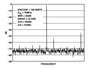
Figure 9. Spectrum:  $f_S = 100$  MSPS,  $f_{IN} = 76$  MHz
