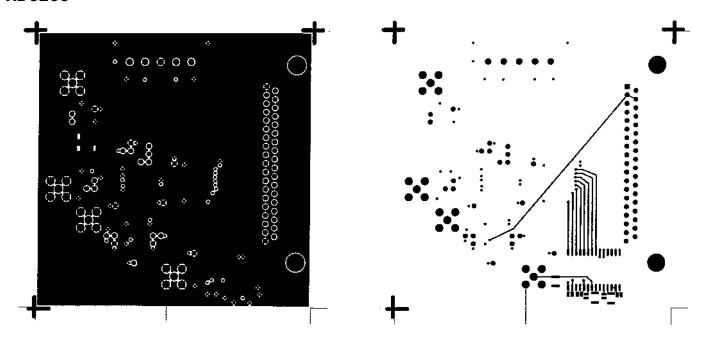
Figure 24. Printed Circuit Board Ground Layer
