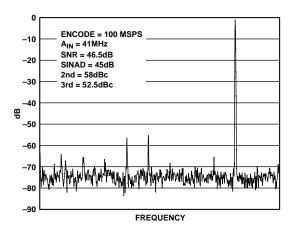
Figure 8. Spectrum:  $f_S = 100$  MSPS,  $f_{IN} = 40$  MHz
