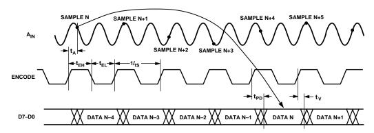
Figure 1. Timing Diagram
