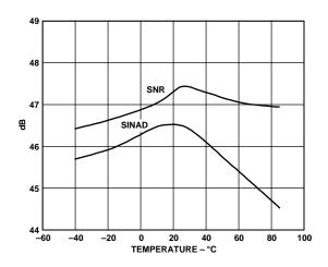
Figure 17. SINAD/SNR vs. Temperature
