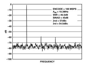
Figure 7. Spectrum:  $f_S = 100$  MSPS,  $f_{IN} = 10.3$  MHz
