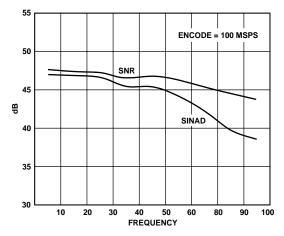
Figure 12. SINAD/SNR vs. A<sub>IN</sub> Frequency
