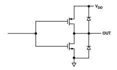
Figure 5. Equivalent Digital Output Circuit
