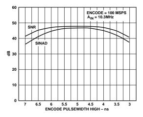
Figure 14. SINAD/SNR vs. Encode Pulsewidth High
