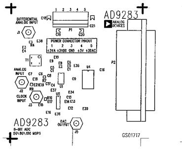
Figure 20. Printed Circuit Board Top Side Silkscreen
