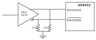
Figure TBD. Using PECL to drive the ENCODE Inputs
