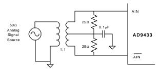
Figure TBD. Transformer-Coupled Analog Input Circuit
