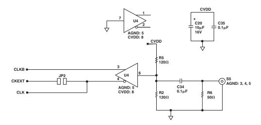
Figure 21. Evaluation Board Schematic: Clock Input
