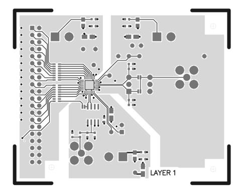
Figure 22. Evaluation Board Layout: Primary Side
