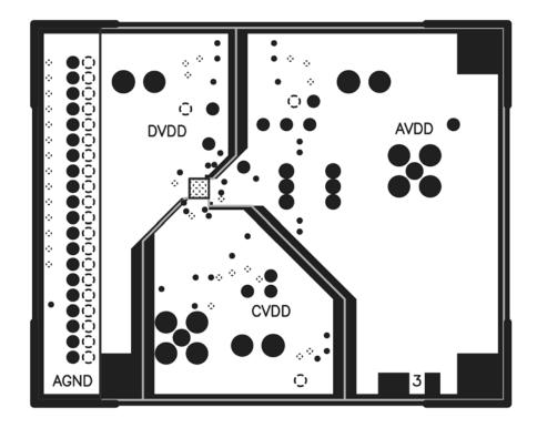
Figure 25. Evaluation Board Layout: Power Plane
