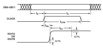
Figure 1. Timing Diagram
