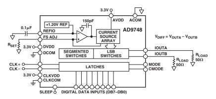
Figure 3. Simplified Block Diagram
