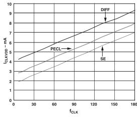
Figure 11. I<sub>CLKVDD</sub> vs. f<sub>CLOCK</sub> and Clock Mode
