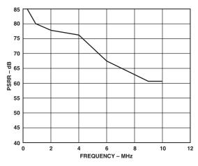
Figure 17. Power Supply Rejection Ratio
