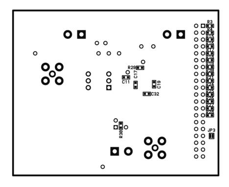
Figure 27. Evaluation Board Layout: Assembly-Secondary Side
