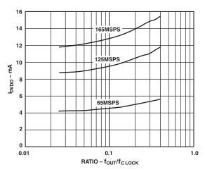
Figure 10. I<sub>DVDD</sub> vs. Ratio @ DVDD = 3.3 V
