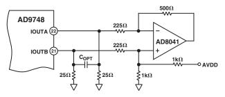
Figure 14. Single-Supply DC Differential Coupled Circuit
