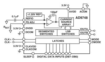
input latches and a 1.2 V temperature compensated band gap reference have been integrated to provide a complete monolithic DAC solution. The digital inputs support 3 V CMOS logic families.
