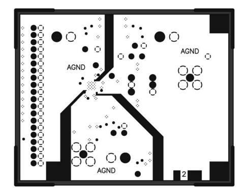
Figure 24. Evaluation Board Layout: Ground Plane
