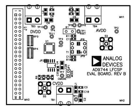
Figure 26. Evaluation Board Layout: Assembly—Primary Side
