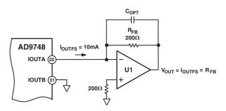
Figure 16. Unipolar Buffered Voltage Output
