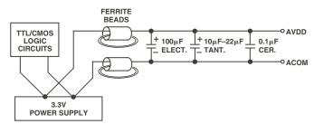
Figure 18. Differential LC Filter for Single 3.3 V Applications
