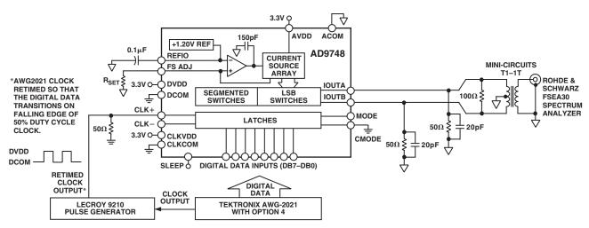
Figure 2. Basic AC Characterization Test Setup
