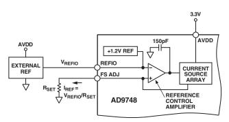
Figure 5. External Reference Configuration
