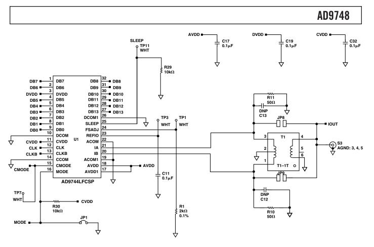
Figure 20. Evaluation Board Schematic: Output Signal Conditioning
