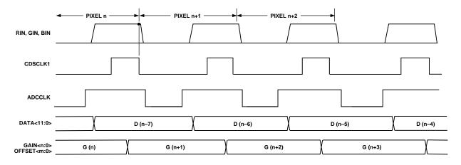
Figure 15. DOUT Latency, 1-Channel SHA Mode
