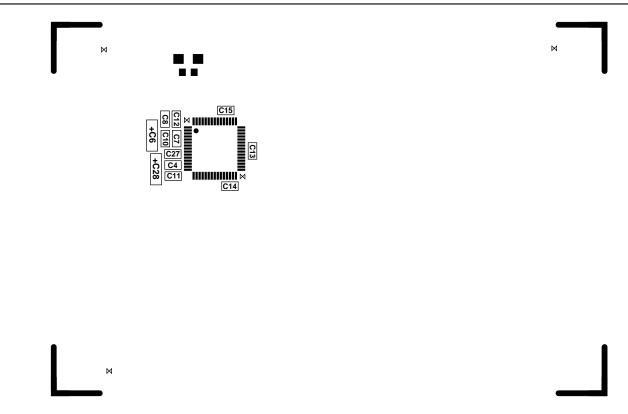
Figure 27. Suggested Capacitor Placement for Single-Side Component Layout
