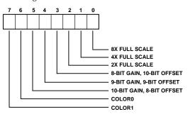
Figure 6. AD9805 Configuration Register Format
