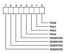
Figure 9. PGA Gain Registers Format
