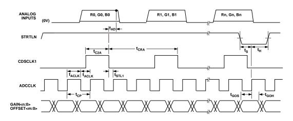
Figure 1b. 3-Channel SHA-Mode Clock Timing
