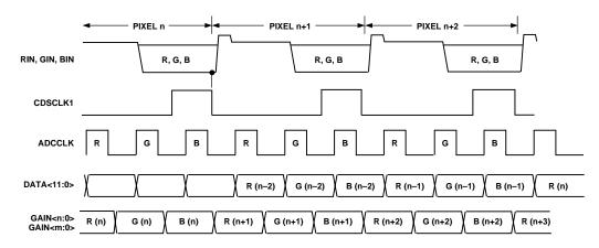
Figure 13. DOUT Latency, 3-Channel SHA Mode
