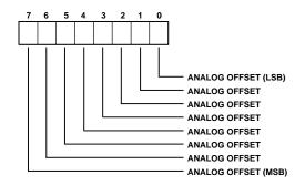
Figure 8. Input Offset Registers Format
