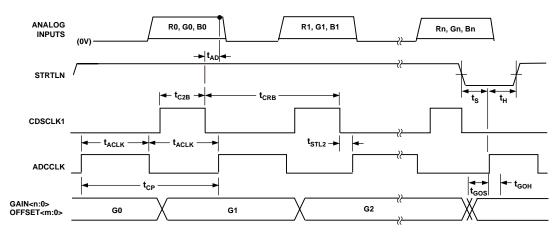
Figure 1e. 1-Channel SHA-Mode Clock Timing (for Blue and Green Channels)
