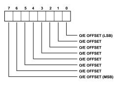
Figure 10. Odd and Even Offset Registers Format
