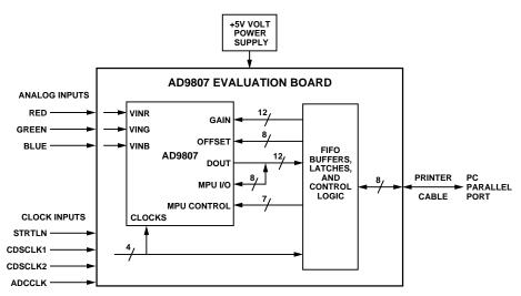
Figure 25. Evaluation System Block Diagram
