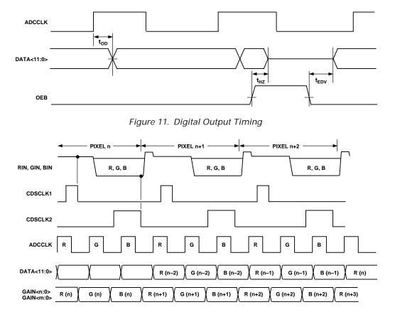
Figure 12. DOUT Latency, 3-Channel CDS Mode
