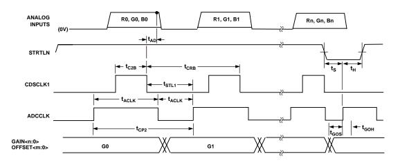
Figure 1f. 1-Channel SHA-Mode Clock Timing (Red Channel)
