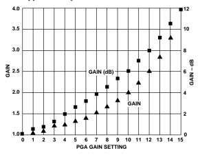
Figure 16. PGA Transfer Function
