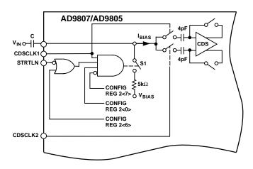
Figure 17. Equivalent Analog Inputs (VINR, VING, and VINB)
