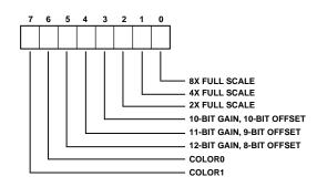
Figure 5. AD9807 Configuration Register Format
