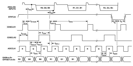
Figure 1a. 3-Channel CDS-Mode Clock Timing
