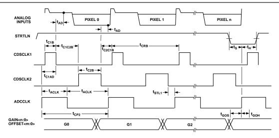
Figure 1d. 1-Channel CDS-Mode Clock Timing (Red Channel)
