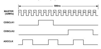
Figure 18. Timing Scheme Using 16 × Master Clock
