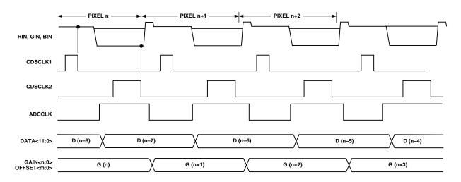
Figure 14. DOUT Latency, 1-Channel CDS Mode
