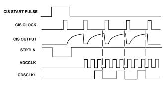
Figure 24. CIS Application Timing Signals
