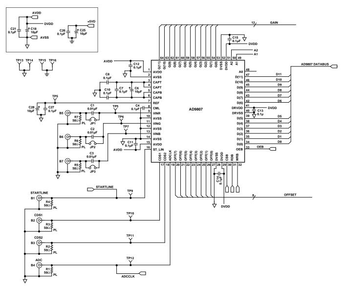
Figure 26. AD9807 Evaluation Board (Digital Circuitry Omitted)
