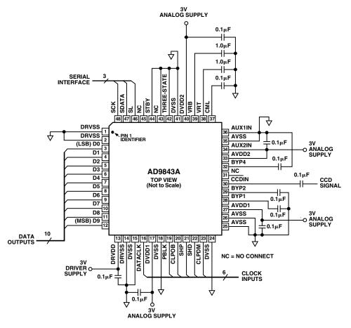
Figure 17. Recommended Circuit Configuration for CCD-Mode
