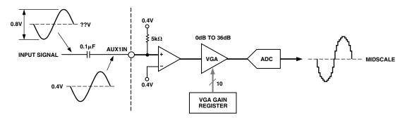
Figure 14. AUX1 Circuit Configuration
