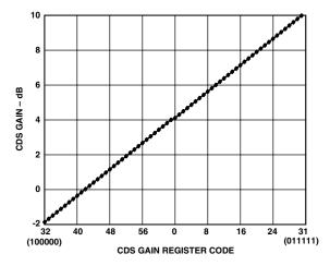
Figure 12. CDS Gain Curve
