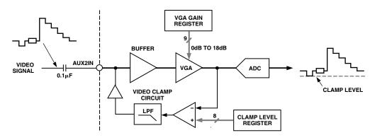
Figure 15. AUX2 Circuit Configuration
