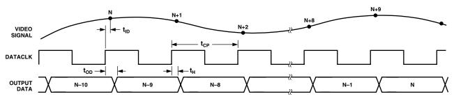
Figure 7. AUX-Mode Timing
