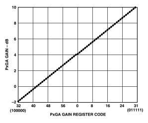
Figure 28. PxGA Gain Curve
