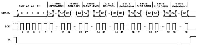
NOTES: 1. ANY NUMBER OF ADJACENT REGISTERS MAY BE LOADED SEQUENTIALLY, BEGINNING WITH THE LOWEST ADDRESS AND INCREMENTING ONE ADDRESS AT A TIME. 2. WHEN SEQUENTIALLY LOADING MULTIPLE REGISTERS, THE EXACT REGISTER LENGTH (SHOWN ABOVE) MUST BE USED FOR EACH REGISTER. 3. ALL LOADED REGISTERS WILL BE SIMULTANEOUSLY UPDATED WITH THE RISING EDGE OF SL.
