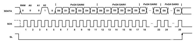
Figure 24. Continuous Serial Write Operation to All PxGA Gain Registers
