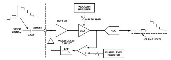
Figure 31. AUX2 Circuit Configuration
