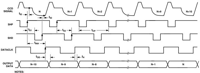
1. RECOMMENDED PLACEMENT FOR DATACLK RISING EDGE IS BETWEEN THE SHD RISING EDGE AND NEXT SHP FALLING EDGE.
