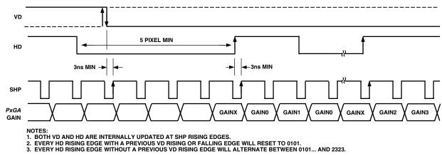
Figure 11. PxGA Mode 2 (Interlace) Detailed Timing
