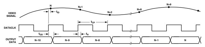
Figure 7. AUX-Mode Timing
