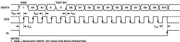
NOTES: 1. RNW = READ-NOT WRITE. SET HIGH FOR READ OPERATION. 2. TEST BITS = INTERNAL USE ONLY. MUST BE SET LOW. 3. SERIAL DATA FROM THE SELECTED REGISTER IS VALID STARTING AFTER THE 5TH SCK FALLING EDGE, AND IS UPDATED ON SCK FALLING EDGES.
