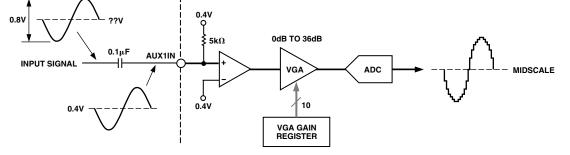
Figure 30. AUX1 Circuit Configuration
