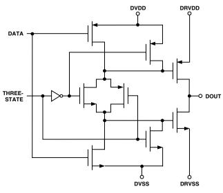
Figure 2. Data Outputs – D0–D11
