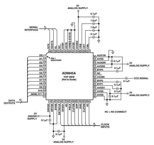
Figure 33. Recommended Circuit Configuration for CCD-Mode
