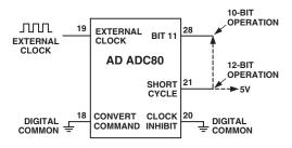
Figure 11. Continuation Conversion with External Clock. Conversion Is Initiated by 14th Clock Pulse. Clock Runs Continuously.
