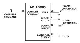
Figure 10. Internal Clock—Normal Operating Mode. Conversion Initiated by the Rising Edge of the Convert Command. The Internal Clock Runs Only During Conversion.
