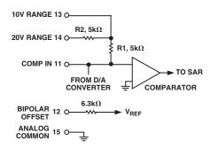
Figure 2. Input Scaling Circuit
