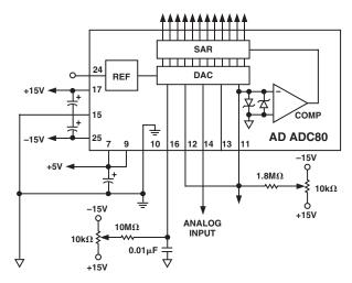
Figure 8. Analog and Power Connections for Bipolar  $\pm\,10$  V Input Range
