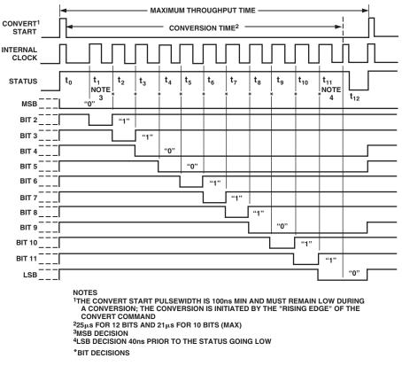
Figure 1. Timing Diagram (Binary Code 011001110110)
