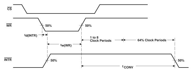
**Figure 2. Write Operation Timing Diagram**
