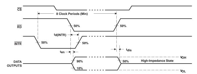
Figure 1. Read Operation Timing Diagram
