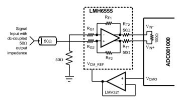
Figure 5. Example of Servoing the Analog Input with  $V_{CMO}$
