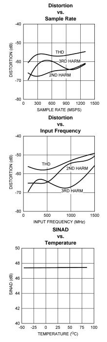
**Typical Performance Characteristics (continued)**  $V_A = V_{DR} = +1.9V$ ,  $f_{CLK} = 1$  GHz (differential clock),  $f_{IN} = 248$  MHz, Differential Inputs, unless otherwise stated. Parameters shown across temperature were measured after recalibration at each temperature.
