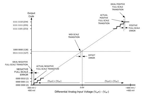
Figure 1. Input / Output Transfer Characteristic
