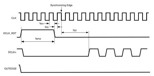
Figure 6. Clock Reset Timing in SDR Mode with OUTEDGE Low
