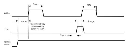
Figure 8. Self Calibration and On-Command Calibration Timing
