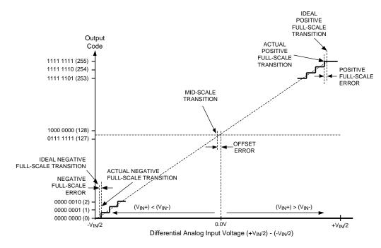
Figure 1. Input / Output Transfer Characteristic
