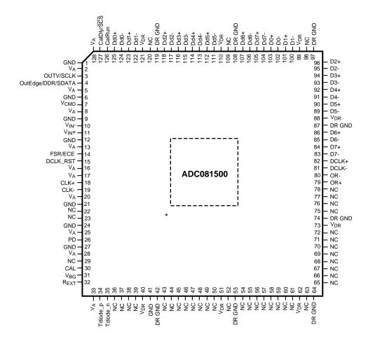
\* Exposed pad on back of package must be soldered to ground plane to ensure rated performance.
