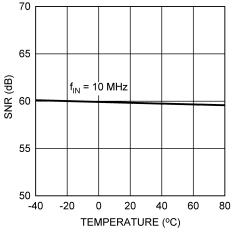
Figure 16. SNR vs. Temperature
