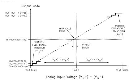
Figure 3. Input vs. Output Transfer Characteristic
