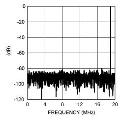
Figure 37. Spectral Response @ 19 MHz Input
