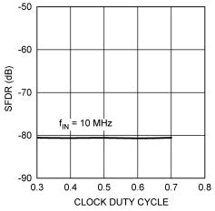
Figure 34. SFDR vs. Clock Duty Cycle
