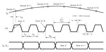
Figure 2. Clock and Data Timing Diagram
