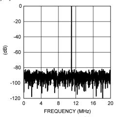
Figure 35. Spectral Response @ 11 MHz Input
