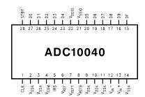
Figure 1. TSSOP Package See Package Number PW0028A
