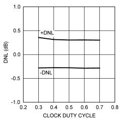
Figure 6. DNL vs. Clock Duty Cycle (DC input)
