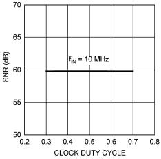
Figure 15. SNR vs. Clock Duty Cycle
