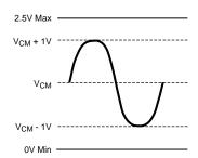
Figure 39. Input Voltage Waveform for a 2V<sub>P-P</sub> Single Ended Input
