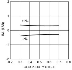
Figure 10. INL vs. Clock Duty Cycle
