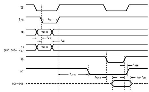
The conversion time (t<sub>CONV</sub>) is set by the internal timer.
