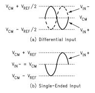
Figure 23. Expected Input Signal Range
