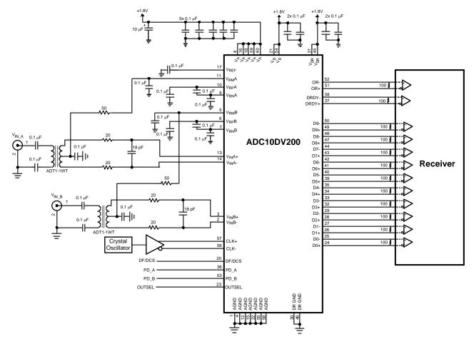
Figure 27. Application Circuit
