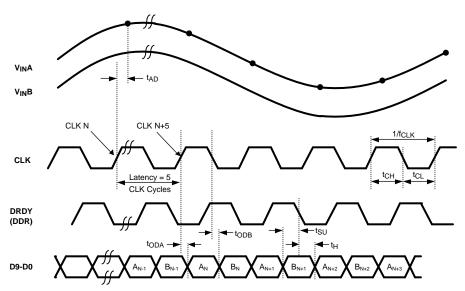
Figure 1. LVDS Output Timing
