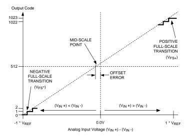
Figure 3. Transfer Characteristic
